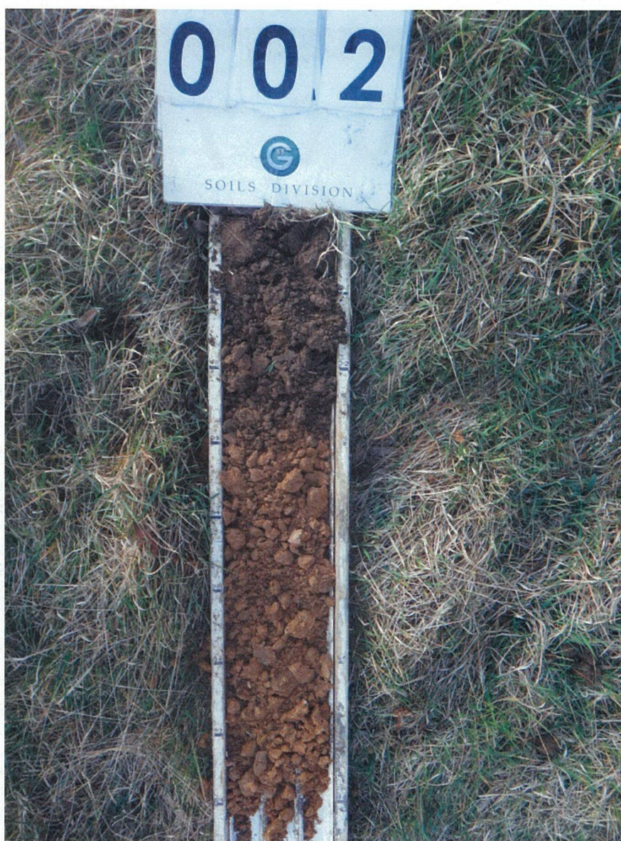
Core 002 – Soil Profile Brown Dermosol
