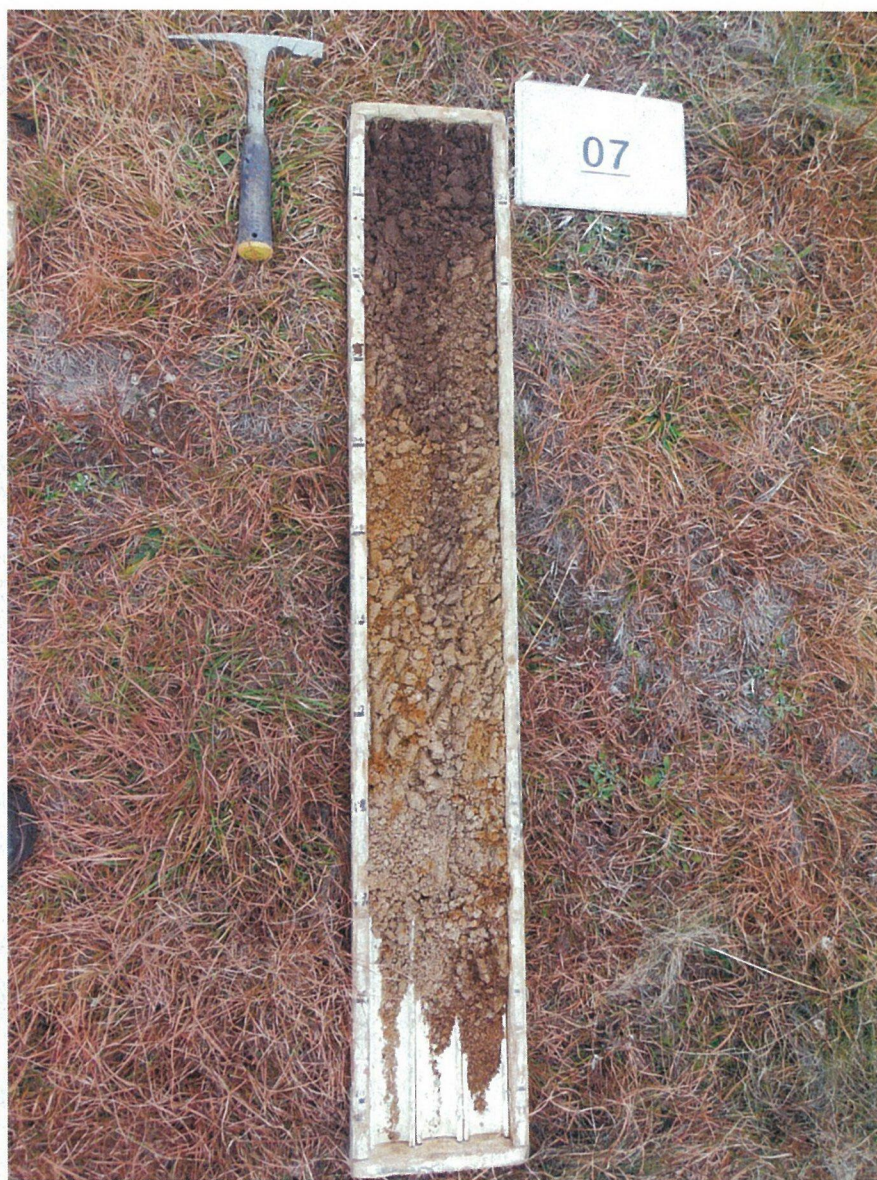
Core 7 – Soil Profile Red Kandosol
