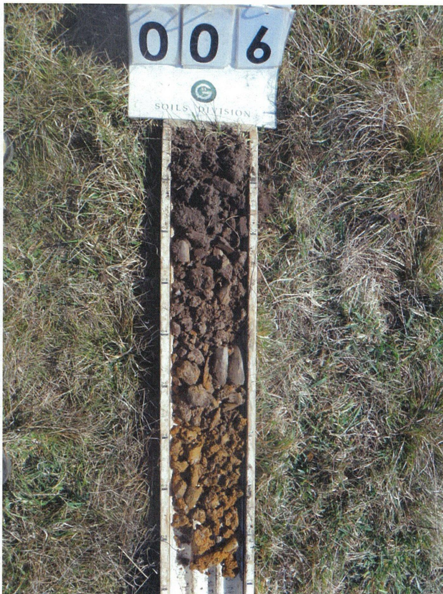
Core 006 – Soil Profile Brown Dermosol
