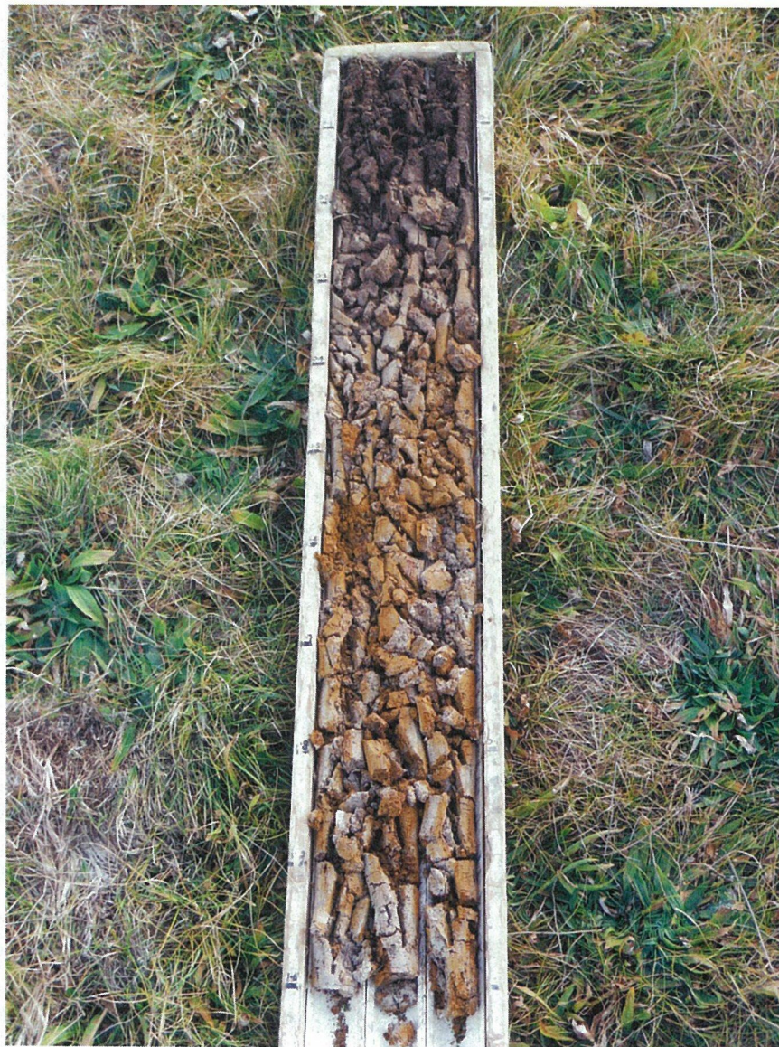
Core 2 – Soil Profile Yellow Chromosol
