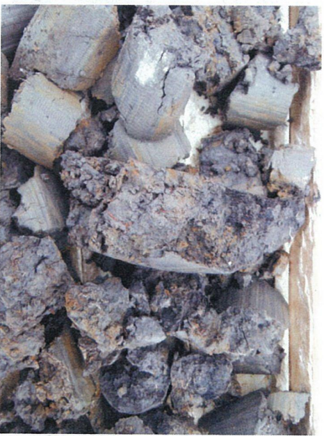
Core 4 – Mottling at 60 cm
