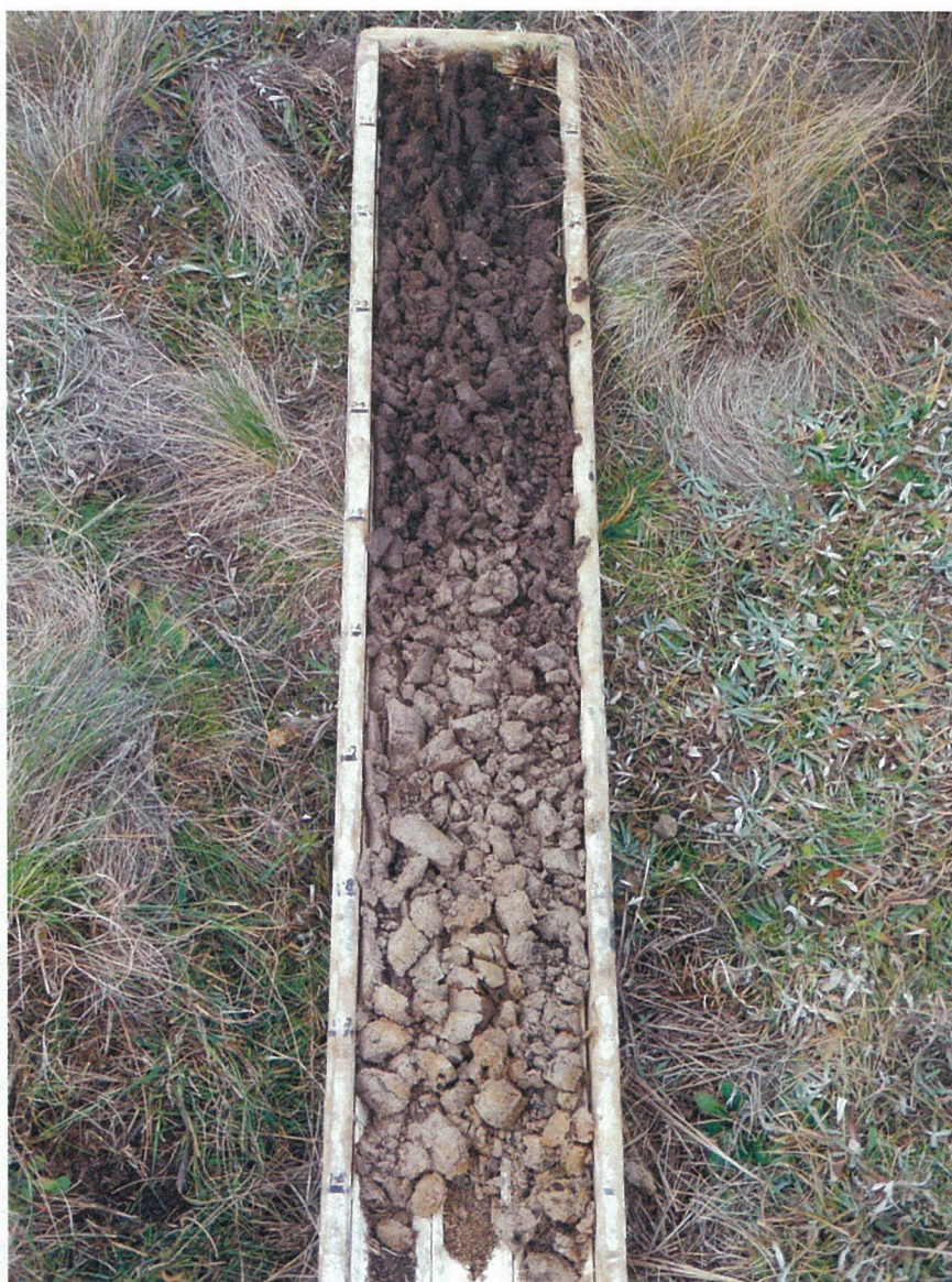
Core 3 – Soil Profile Grey Chromosol
