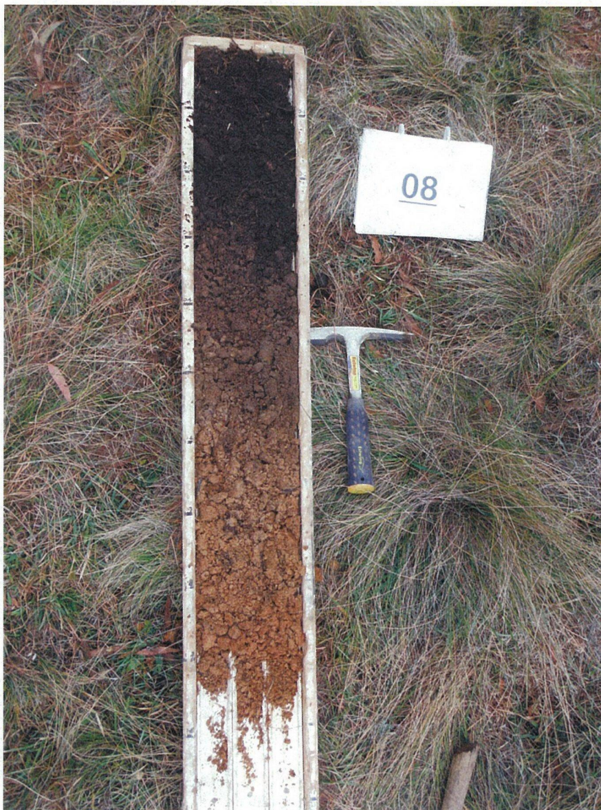
Core 8 – Soil Profile Brown Kandosol
