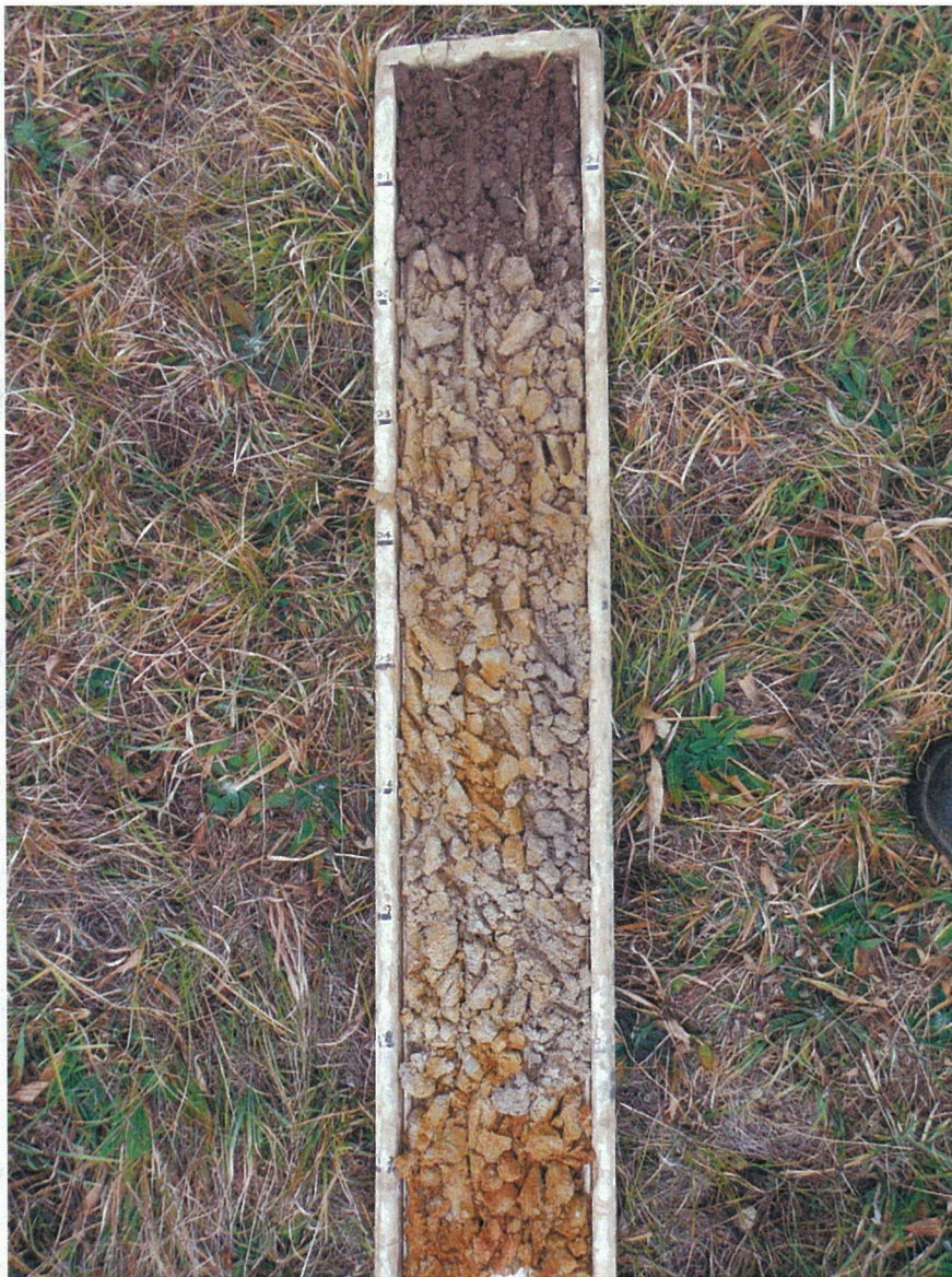
Core 5 – Soil Profile Red Dermosol
