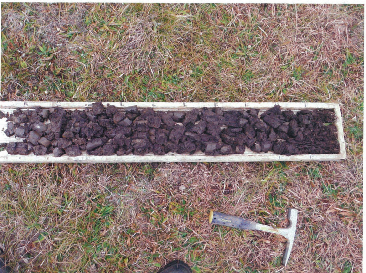
Core 4 – Mottling at 60 cm
