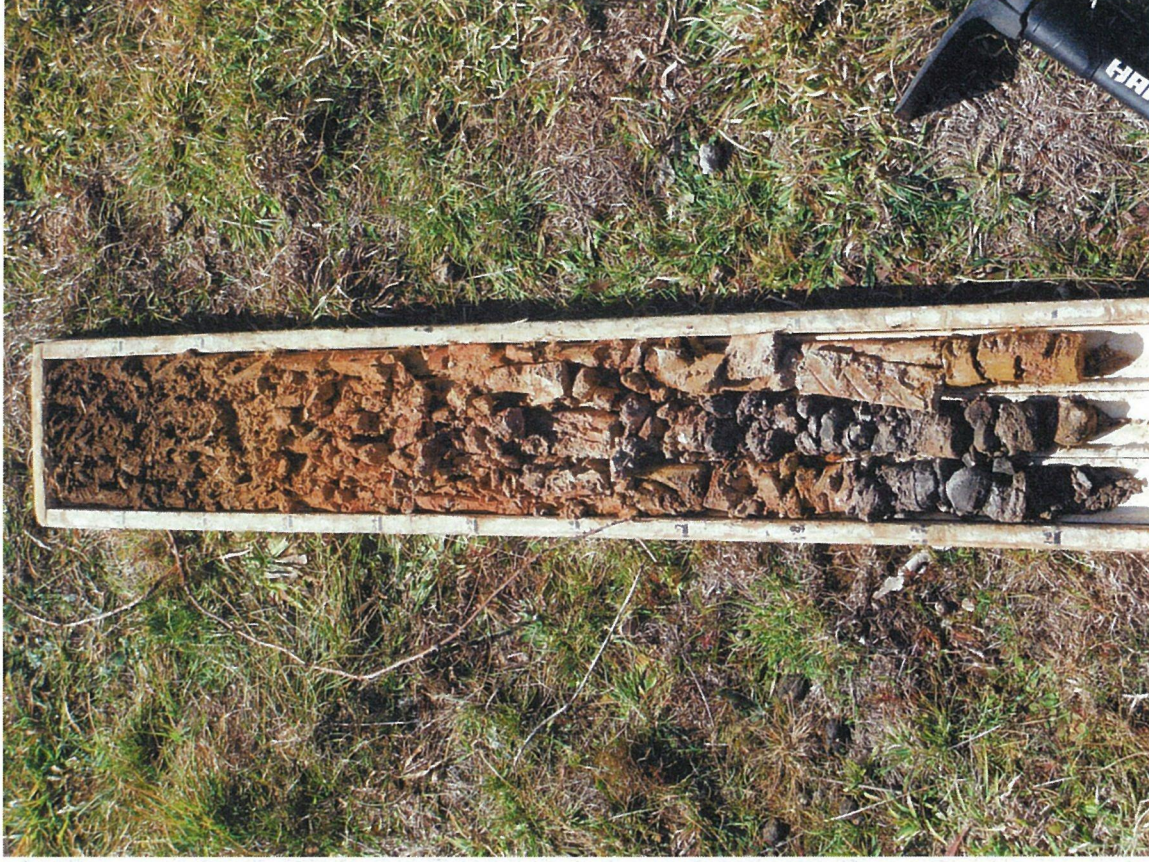
Core 1 – Soil Profile Yellow Chromosol
