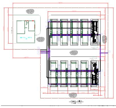
The conceptual design portrays the main treatment components for a desalination plant of 15,000 m3/day, comprised of 10 NIROBOX SW-MEGA units, or 30,000 m3/day, with two arrays of the above. The proposed will be offered not including the intake, storage tanks, distribution unit and discharge system.
