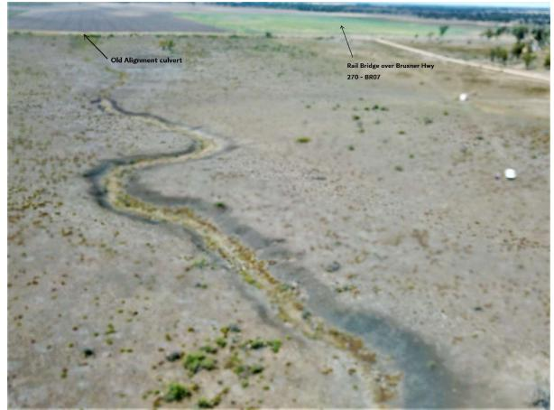
This erosion has emanated from flood shadowing as described by Dr Loch. The paddock in which the erosion is occurring is native perennial grassland, classified as a critically endangered ecological community under the Federal EPBC Act. <u>This erosion must be</u> repaired by ARTC as part of this project or further significant and catastrophic erosion will occur in this paddock. (photo below Gully from Whalan Creek)
