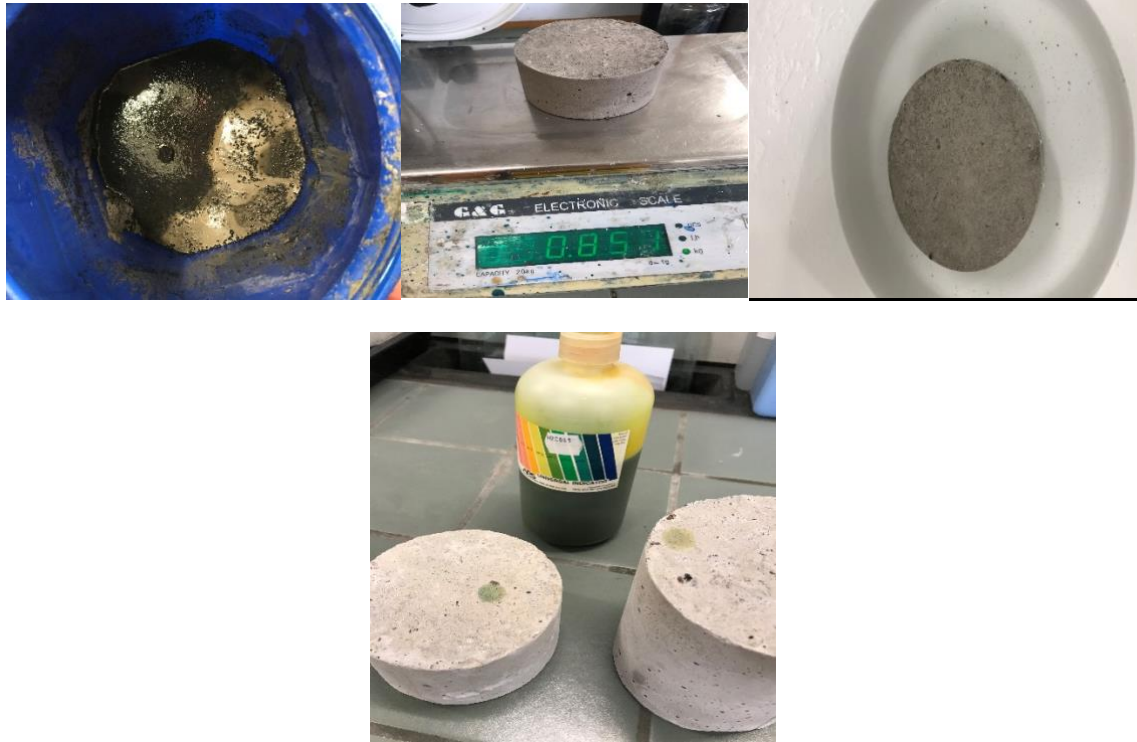
Figure 1 Loy Yang B Brown Coal bottom Ash before and after submersed in water for 30days with no physical changes, preliminary, universal indicator tests presents a neutralized PH level between 6-7.
