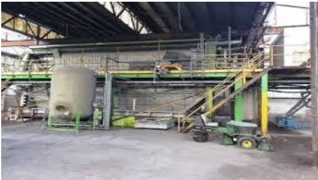
GHT 1500 Filter Press, can be mobilised from storage facility in Geelong Victoria to facilitate the remediation of ash ponds and beneficial reuse of ash at Bayswater Power Plant .
