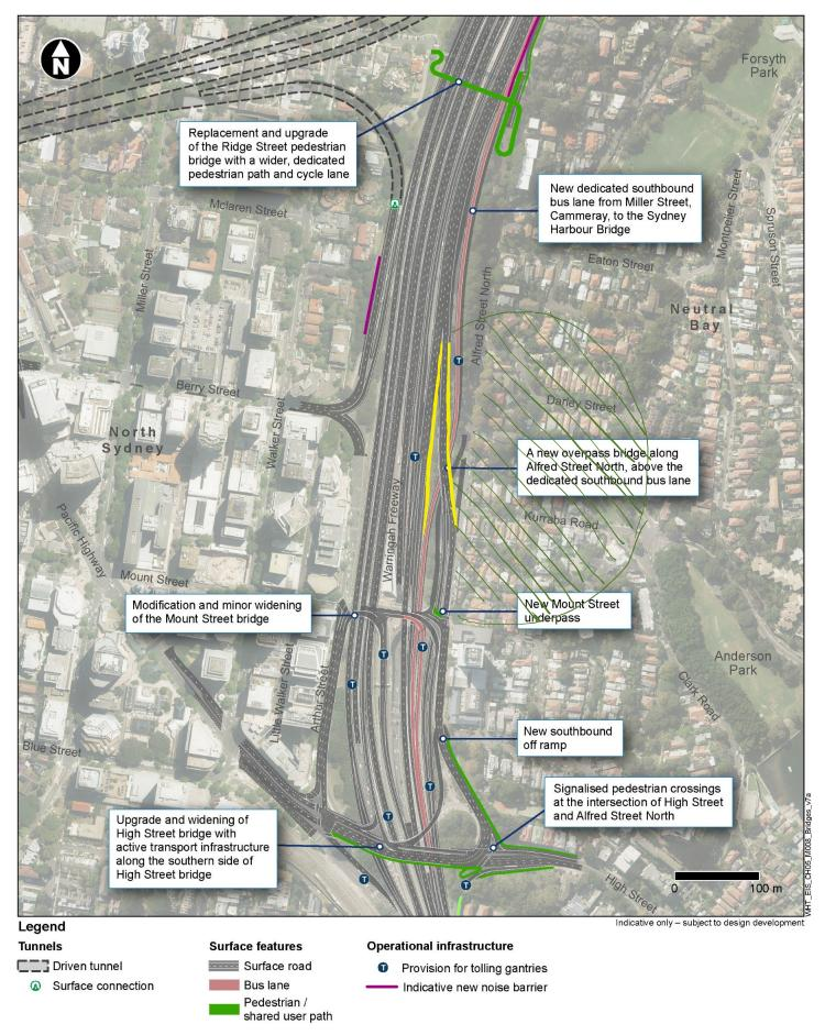
Figure 5-28 New, modified and relocated road bridges of the Warringah Freeway Upgrade component (map 1)
