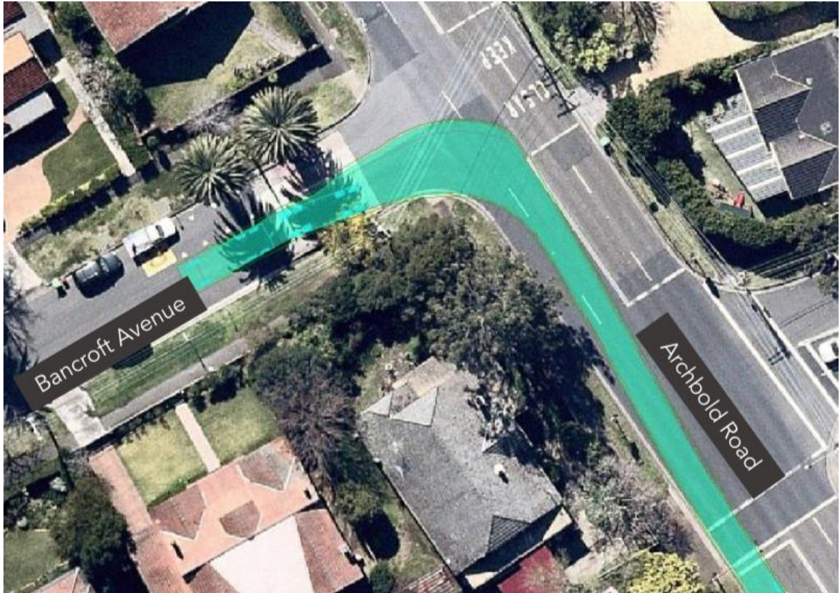
Fig. 2 - Turning circle – Archbold to Bancroft
