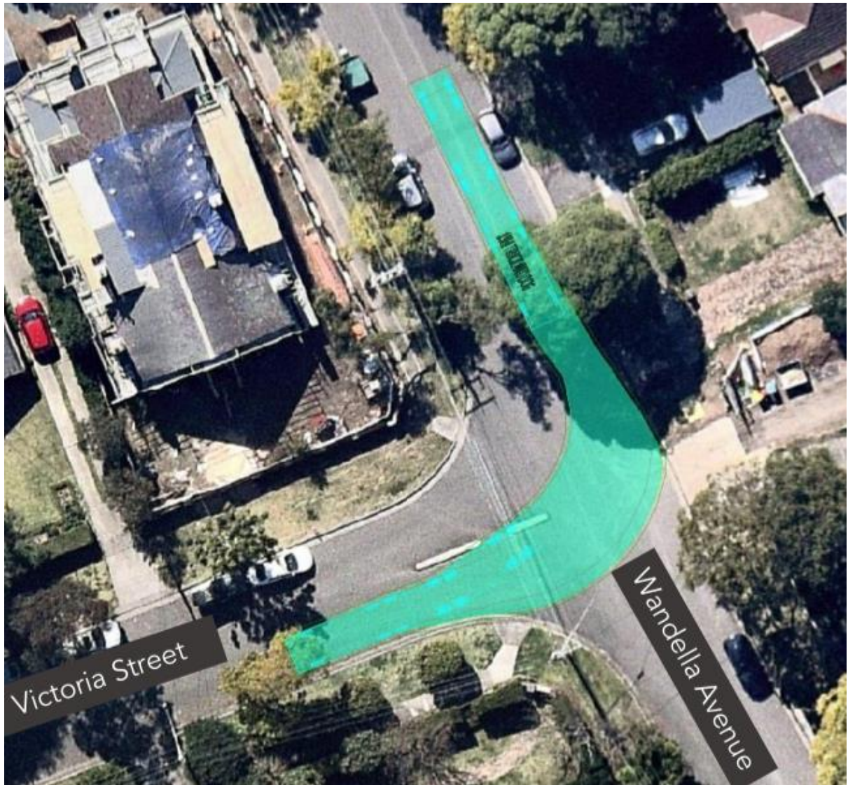
Fig. 4 - Turning circle – Wandella to Victoria
