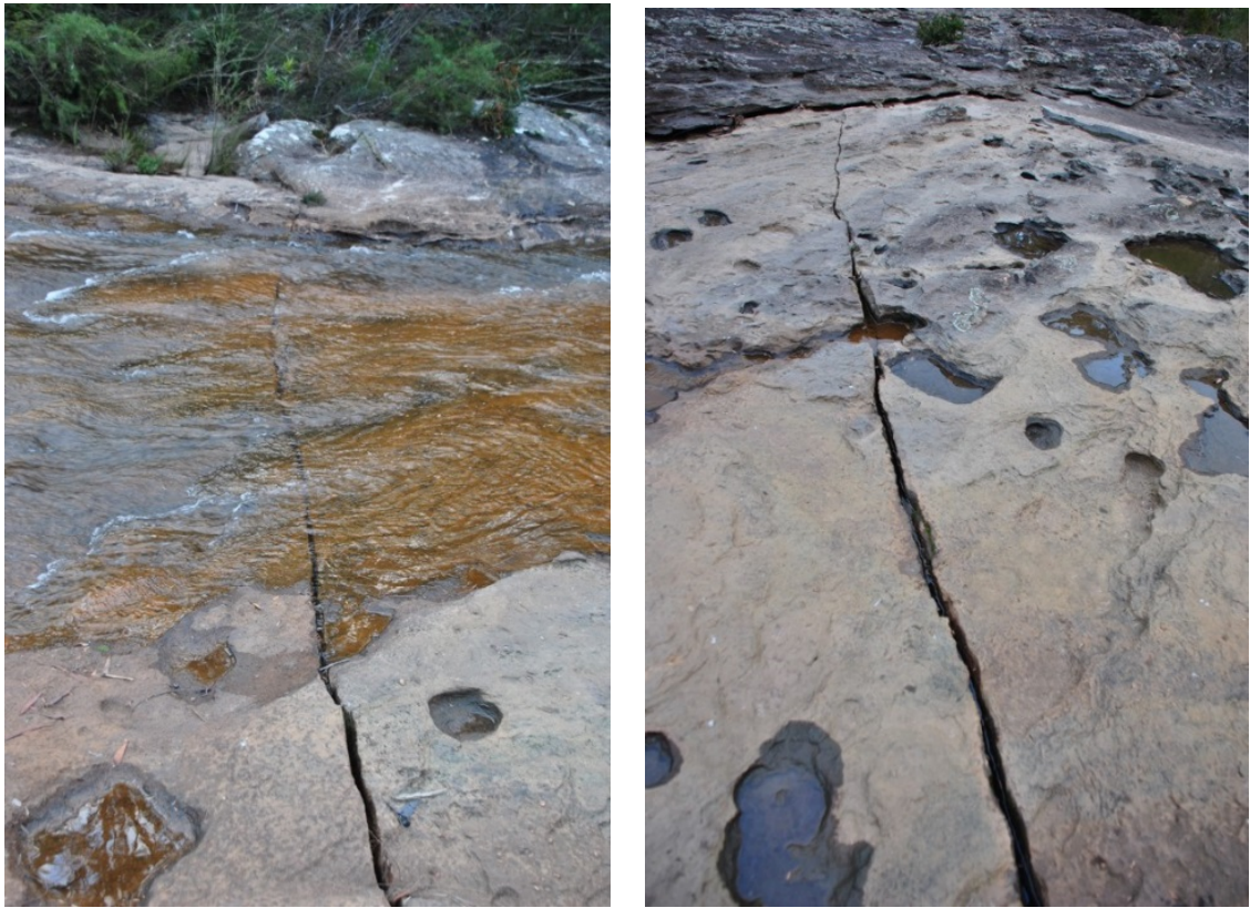
Figure 1 Evidence of long wall mining induced cracking from subsidence on the left bank (left) and right bank (right) at Waratah Rivulet (WR4), Woronora (April 2015)
