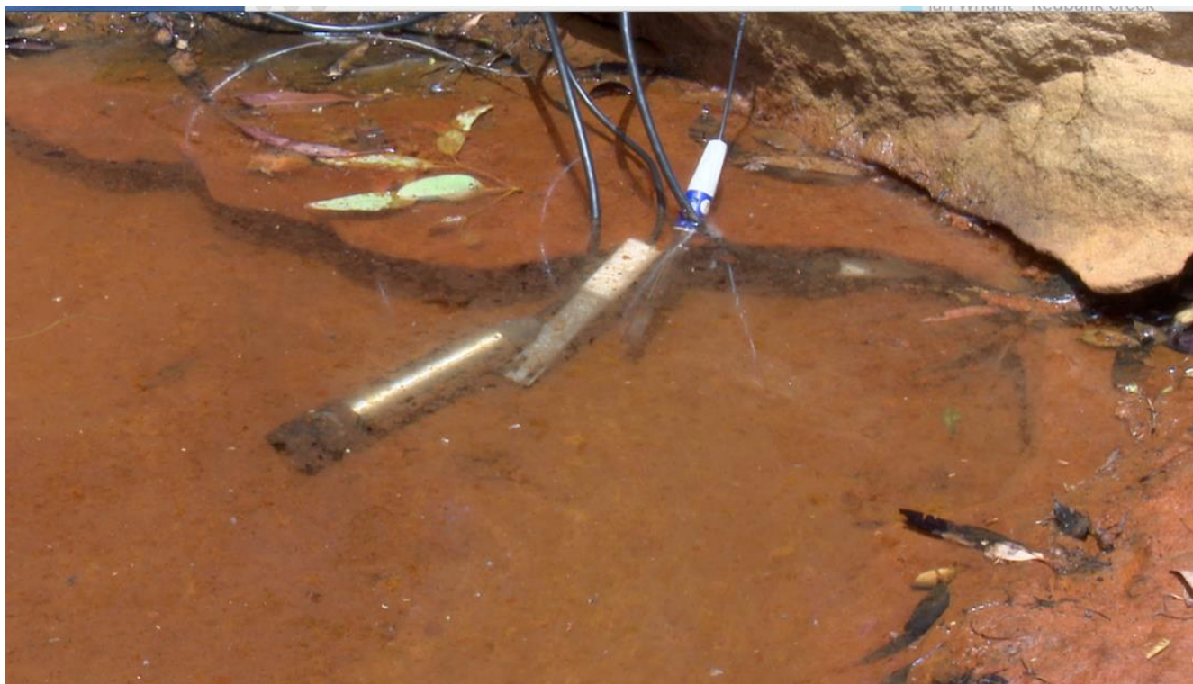
Picture 3: Severe subsidence fracturing of Redbank Creek, near Picton. This was the site of a ground water ‘vent’ where upwelling groundwater flowed into Redbank Creek, through a fresh subsidence fracture. Water quality was extremely poor for the aquatic ecosystem with very low dissolved oxygen, very high salinity, and hazardous concentrations of metals, such as zinc and nickel (Morrison et al. 2018; Morrison et al. 2019).
