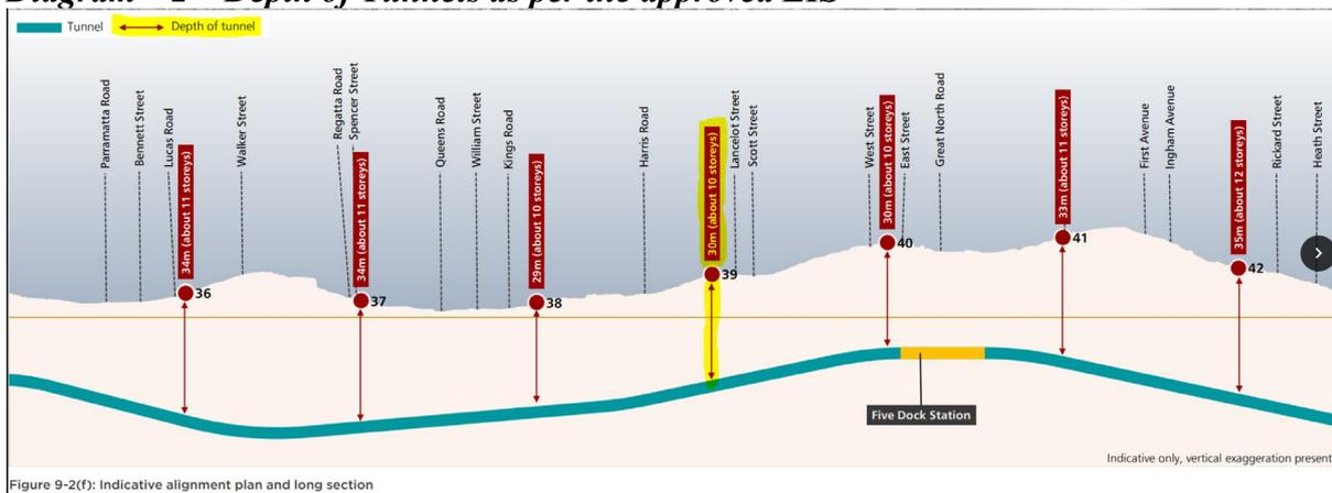
FDPS P&C requests that the tunnel depths under the school are consistent with the original EIS at 30m as per Diagram 2 above, versus the updated 23 metres in Diagram 1.
