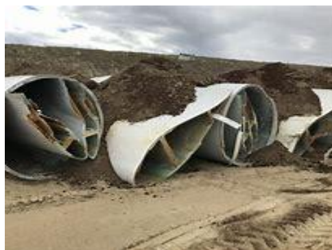
Disposing of cutup wind turbine blades
