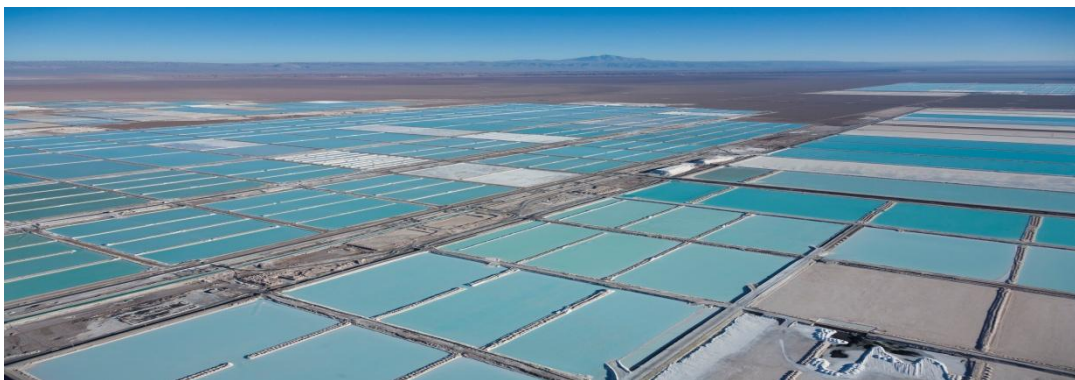
Extraction of lithium pumped from underground salar brine deposits into evaporation ponds
