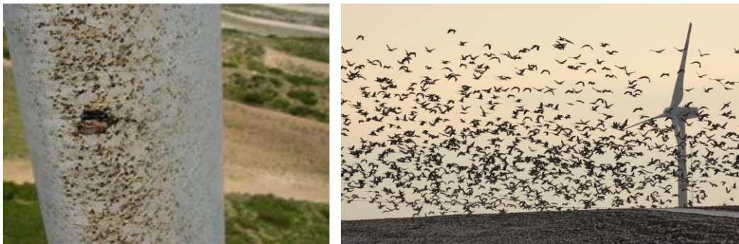
The build up of dead insects reduces the output. Insects attract birds. Blade tip speed can exceed 280kmph
