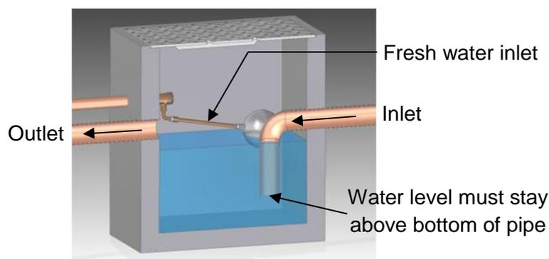
**Figure 56 - Example flame trap**
