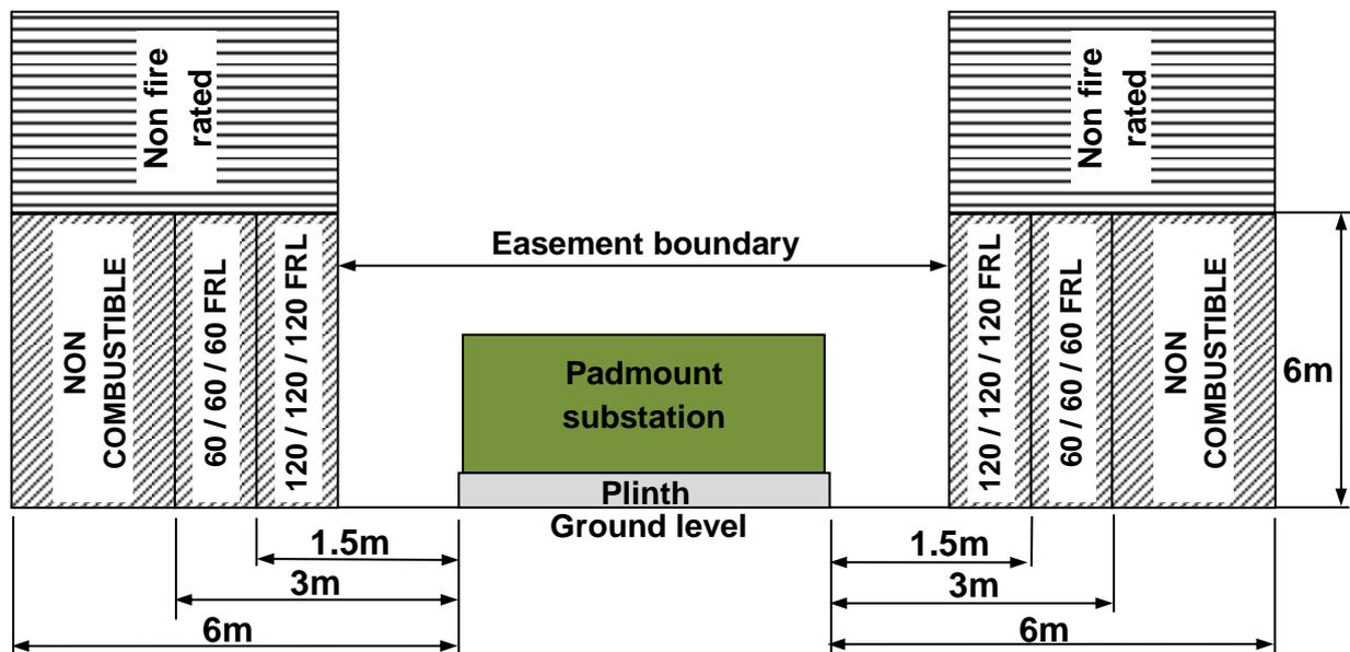
Figure 45 - Minimum FRL clearances for components
