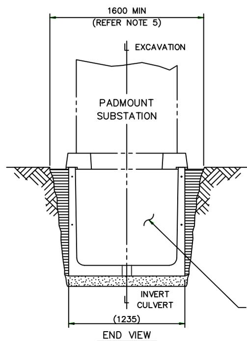
BARRIERS ARE PROVIDED AT BOTH ENDS OF THE INVERT CULVERT AND SAND BAGGING IS REQUIRED TO SEAL THE OPENINGS LEFT FOR CABLE ACCESS THUS PREVENTING THE INGRESS OF BACKFILL.
