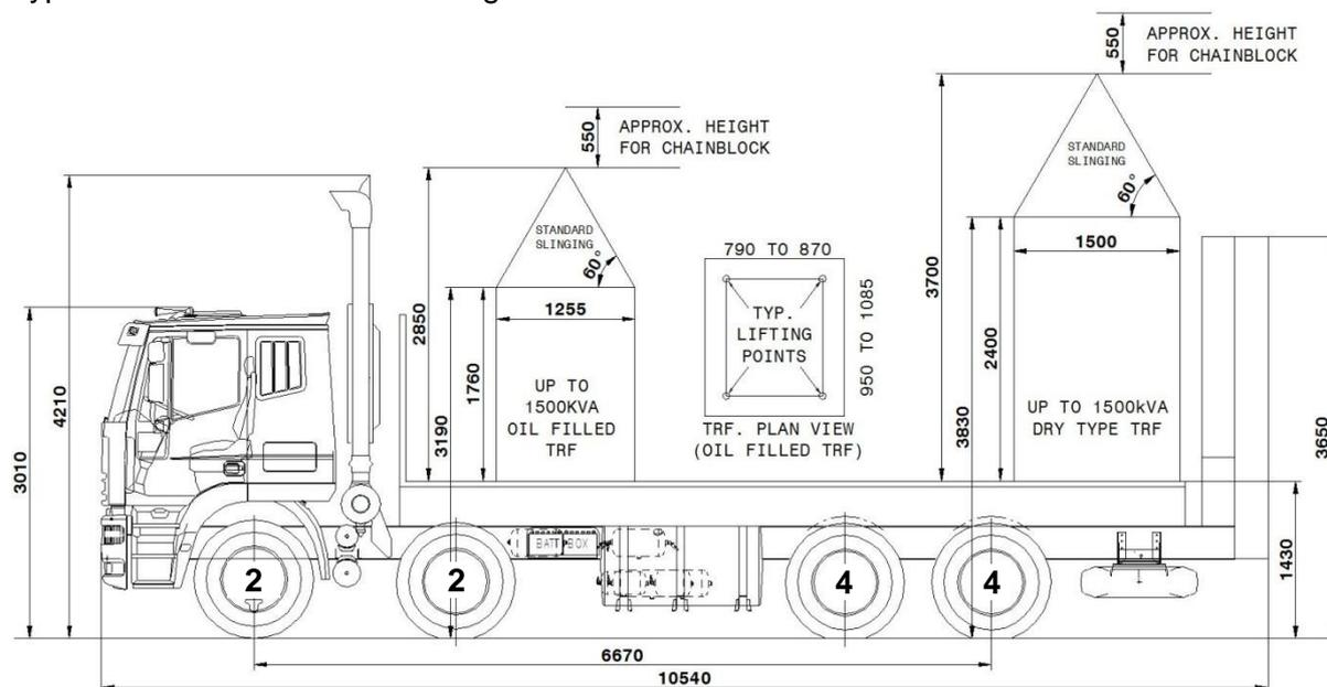
Figure 33 - Truck detail - Type 1
