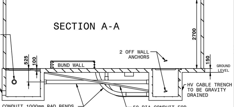
125 DIA CONDUIT 1000mm RAD BENDS. LV STREET SUPPLY AND TO HV END OF TRANSFORMER, TO BE BELLMOUTHED
