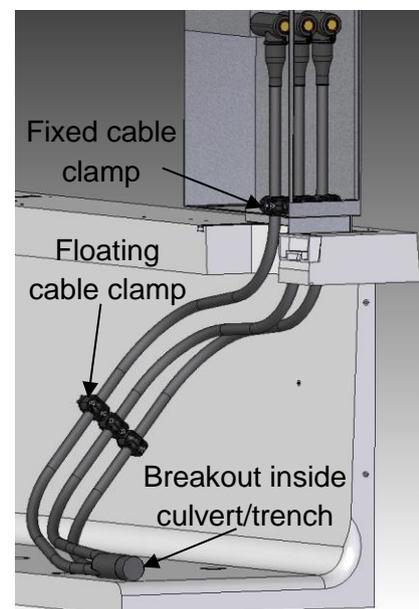
**Figure 38 - Typical cable breakout**
