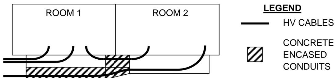
Figure 55 - Typical protected cable detail for multiple rooms
