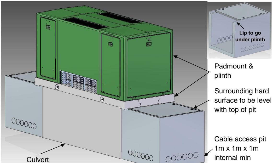
Figure 50 - Example substation with access pits
