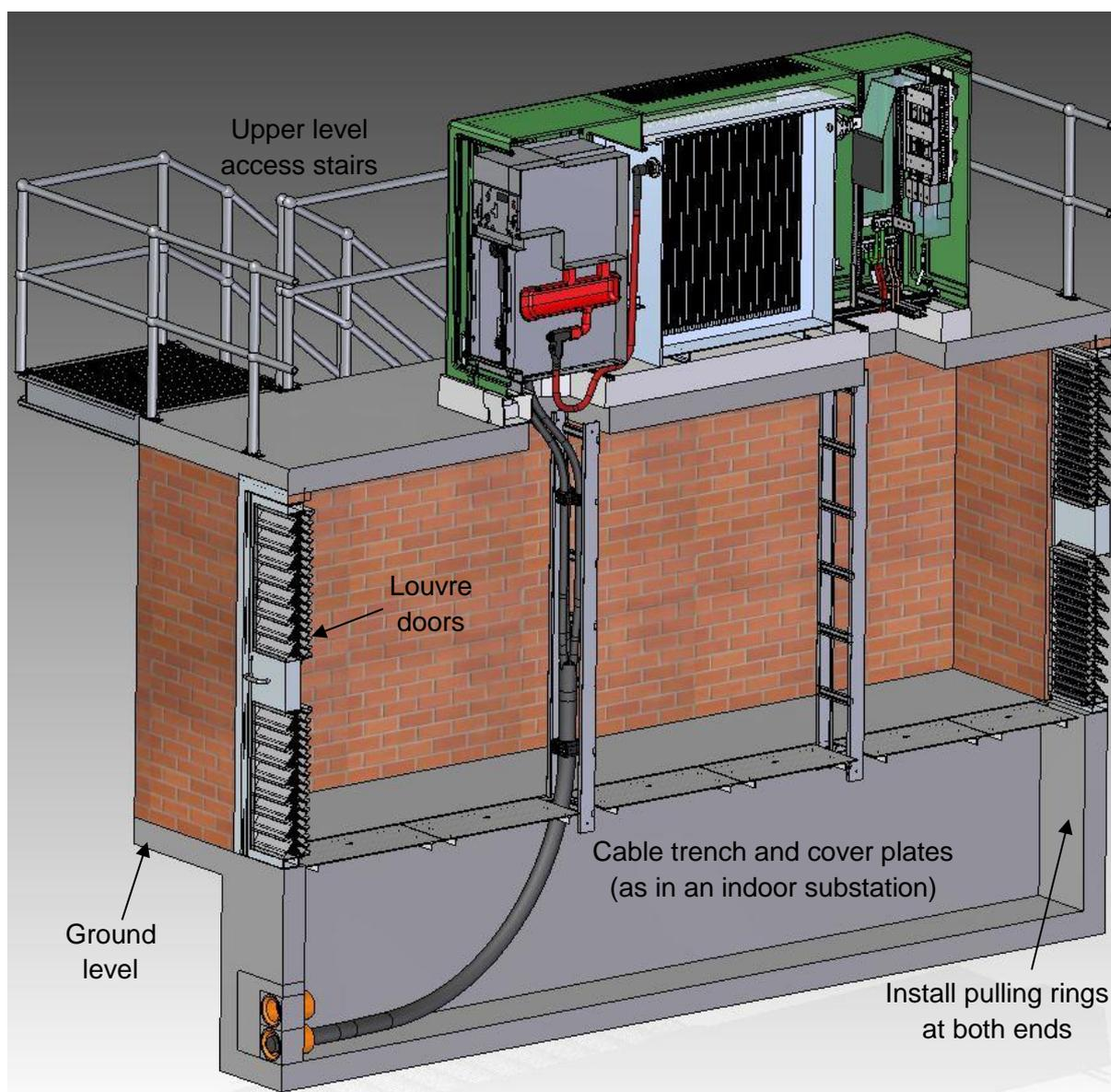
**Figure 52 - Section view of example raised sub**
