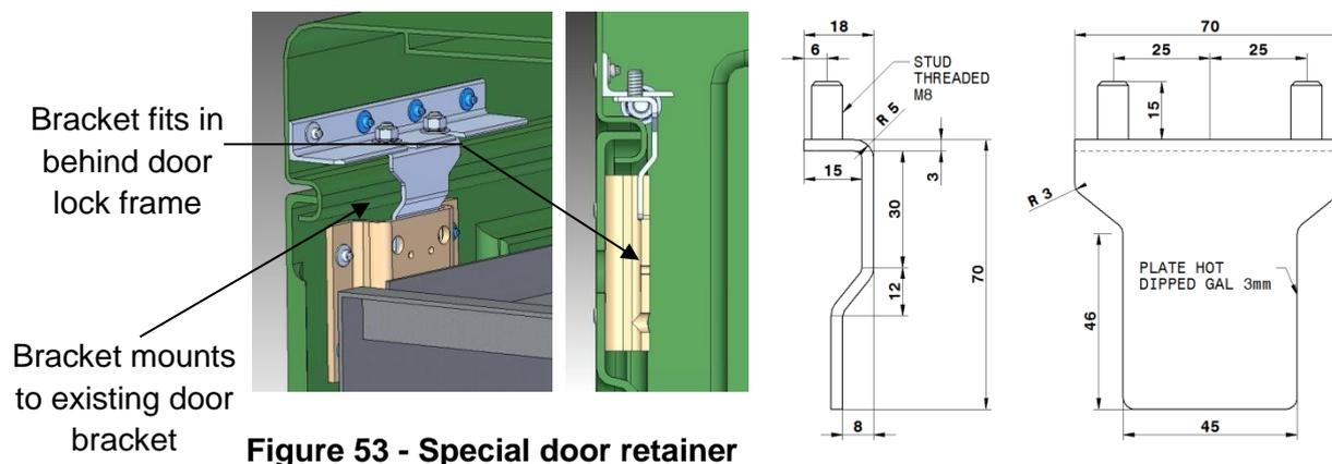
**Figure 53 - Special door retainer**
