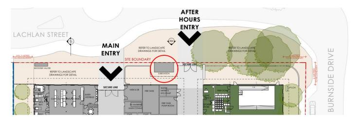
From Endeavour Energy's perspective the fact that provision is being made for a padmount substation is a positive. Endeavour Energy's general requirements is for a padmount substation to be at ground level and have direct access from a public street (unless provided with appropriate easements for the associated underground cables and right of access).
