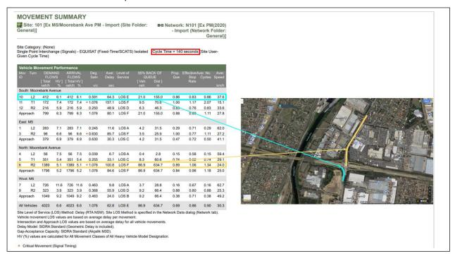
The first impression is that the cycle time of 140 seconds is highly unlikely to be accepted by the TfNSW. The traffic engineers would certainly be happier with a smaller cycle time,
