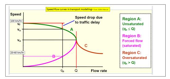
If we only know the Flow rate, say qa, from the graph, the speed could either be on the green line, (Region A, Unsaturated) or on the pink line (Region B, Forced Flow, with a much slower speed, because of congestion).
