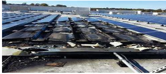
PV solar panel fire result
