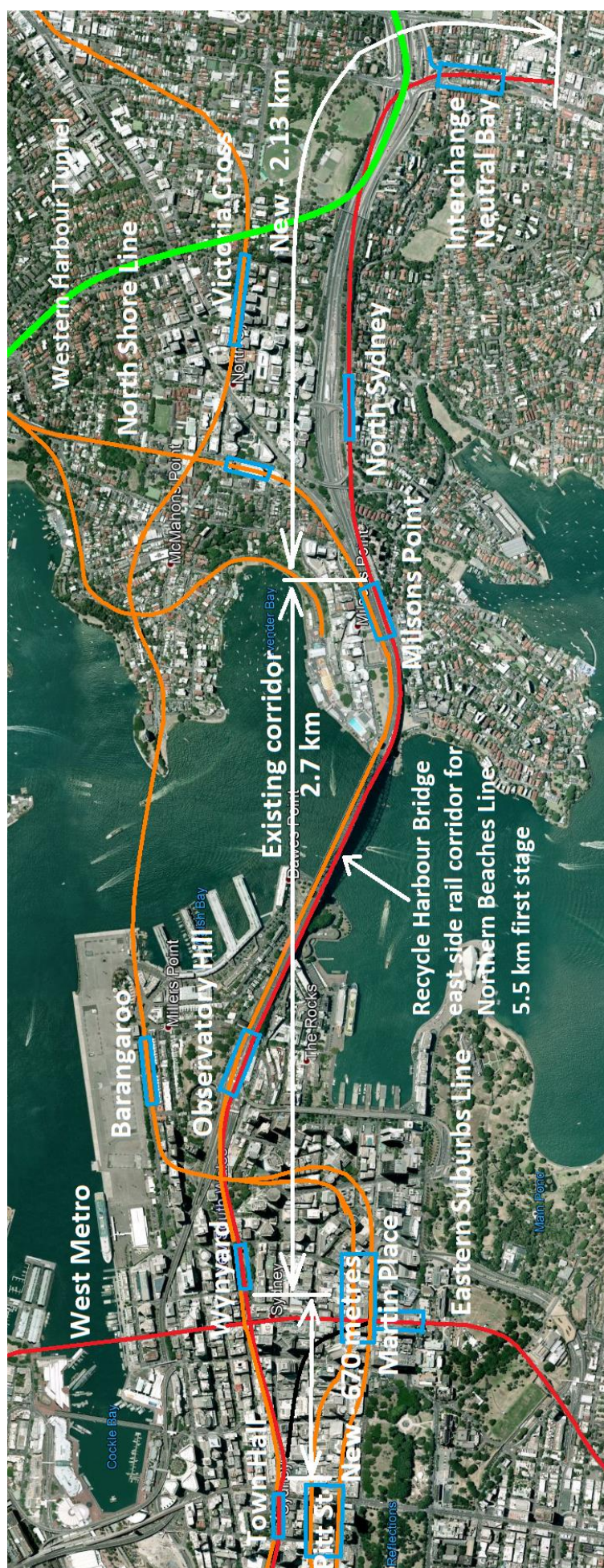
Figure 3.3.5.2 – Six-lane WHT permits rededication to rail of the former Harbour Bridge rail (tram) corridor from Wynyard to Milsons Point with an underground extension to Neutral Bay
