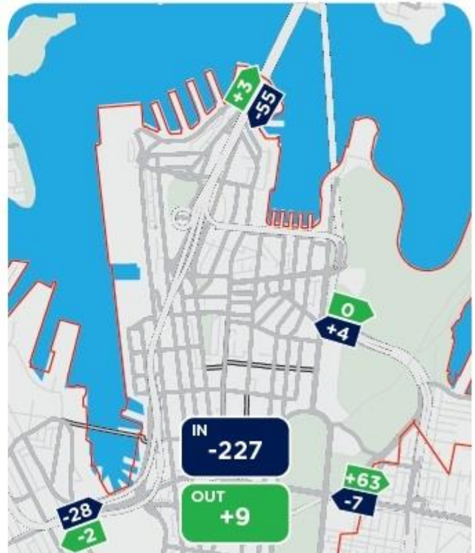
Figure 3.3.5.1 – 2011 buses crossing harbour Bridge in AM peak hour (379 buses), and proposed diversion to Cahill Expressway (55 buses)
