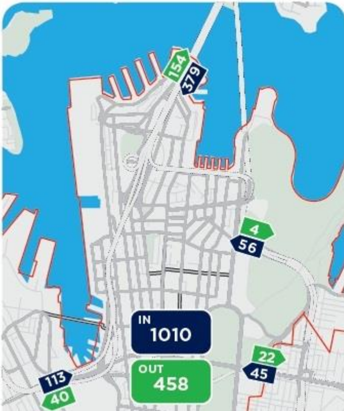
Figure 3.3.5.1 – 2011 buses crossing harbour Bridge in AM peak hour (379 buses), and proposed diversion to Cahill Expressway (55 buses)
