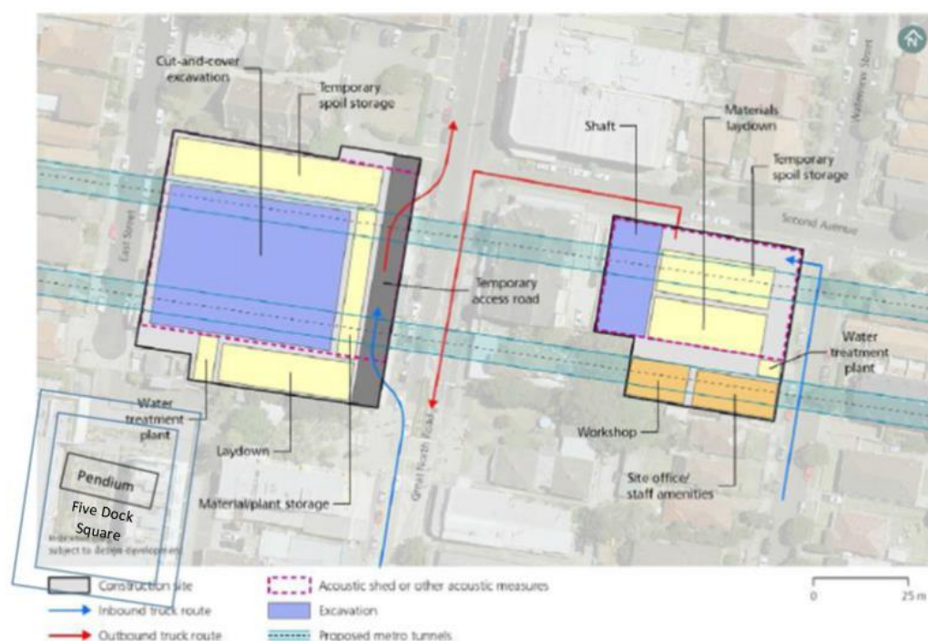
Figure 9-28: Five Dock Station indicative construction site layout
