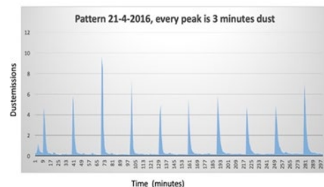
Figure 7: Most of the time, bypassing (dump stacks) takes only a few minutes
