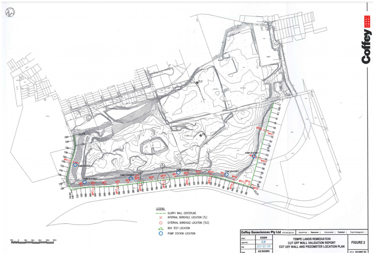
Figure 4-2 Monitoring wells and leachate pump pits located along the bentonite wall
