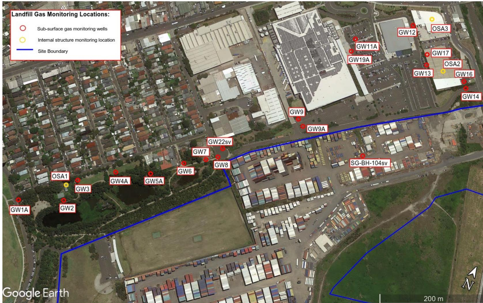
Figure 1: Monthly offsite landfill gas monitoring locations
