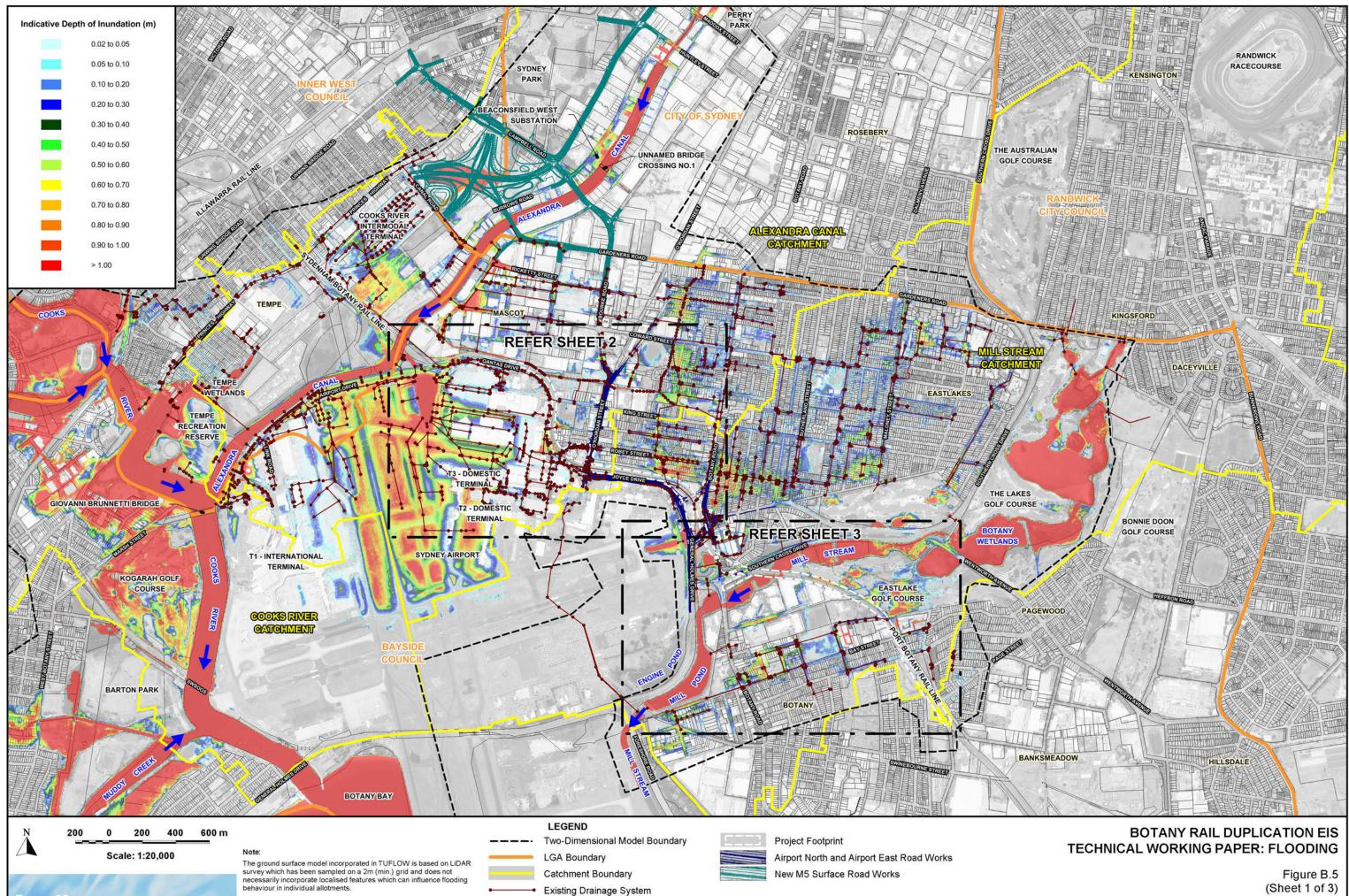
Figure B.5 (Sheet 1 of 3) PATTERNS OF MAIN STREAM FLOODING AND MAJOR OVERLAND FLOW PRE-PROJECT CONDITIONS - 0.2% AEP EVENT
