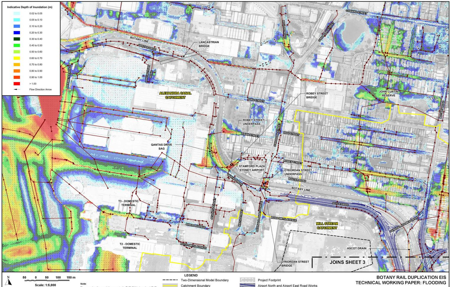
The ground surface model incorporated in TUFLOW is based on LiDAR survey which has been sampled on a 2m (min.) grid and does not necessarily incorporate localised features which can influence flooding behaviour in individual allotments.
