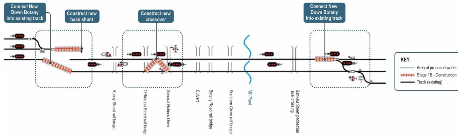
Figure 7.4 Indicative construction staging – Stage 1B: Cut over and head shunt
