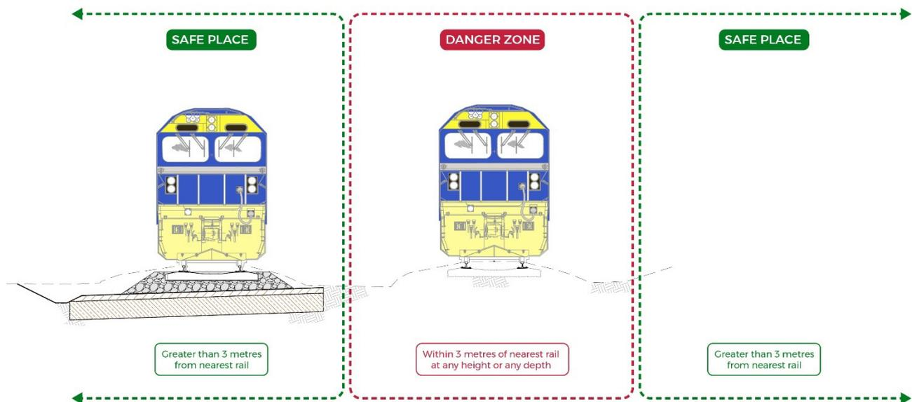
*Note: The above diagram illustrates the potential danger zone where the rail track on the right is the live/active rail corridor while the track on the left hand side is being constructed.*
