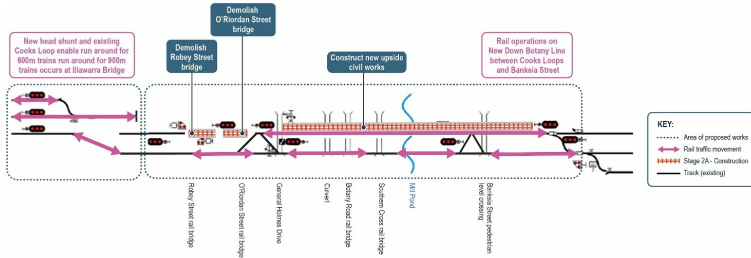
Figure 7.5 Indicative construction staging – Stage 2A: Demolish existing O’Riordan Street and Robey Street bridges
