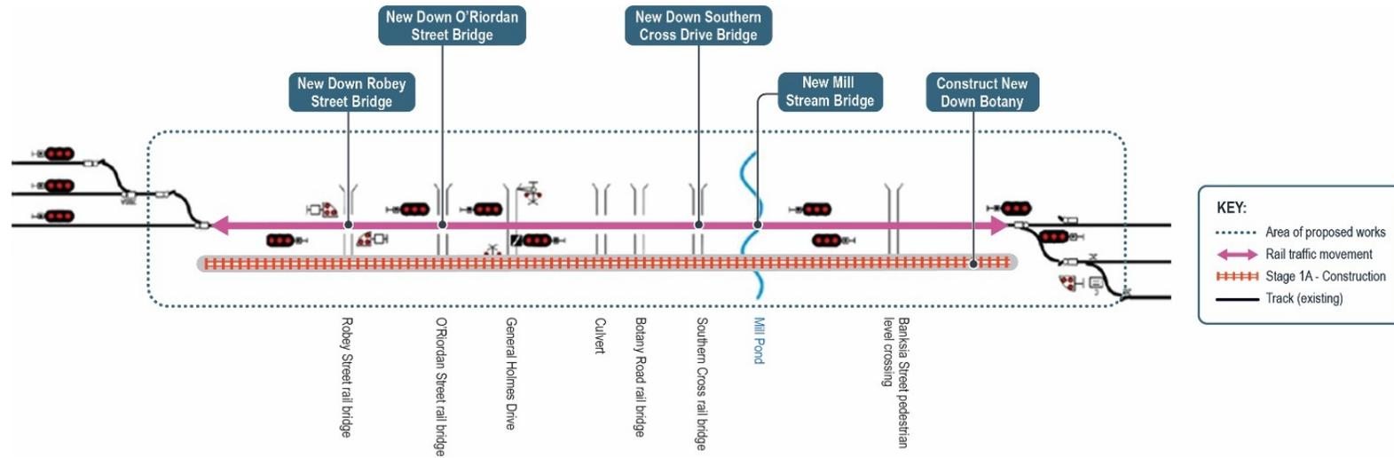
Figure 7.3 Indicative construction staging – Stage 1A: Construction of new down Botany Line
