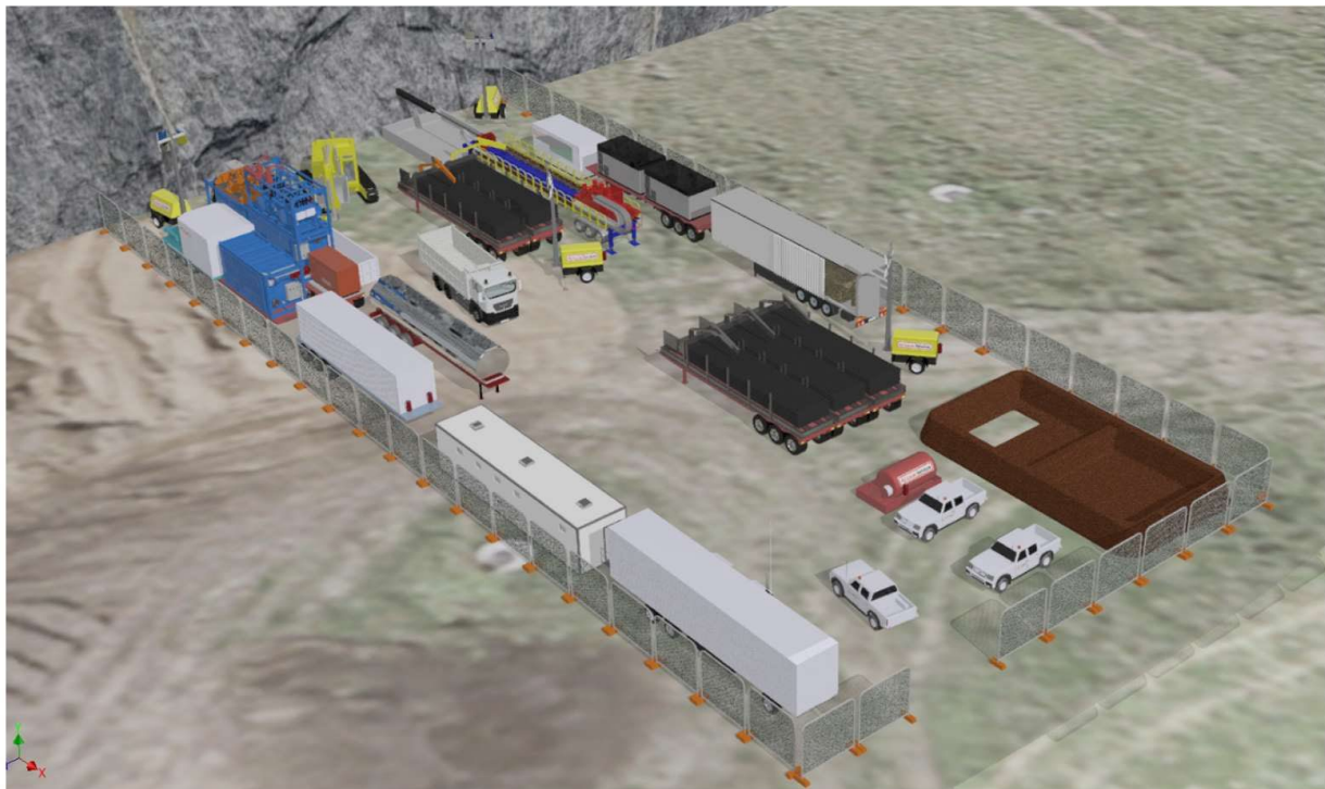
Figure 2.5 Artist impression of the example drill site layout (source: FGJV)
