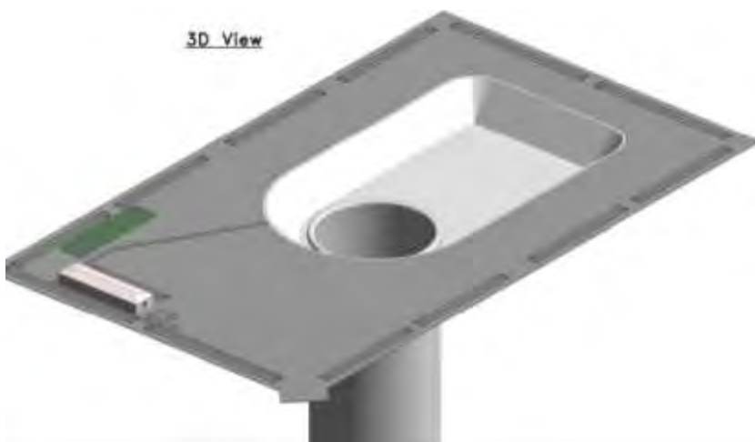
Figure 3.26 3D view of alternative surge shaft design
