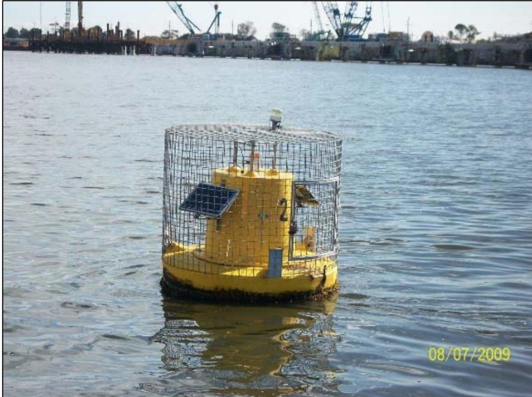
*Photograph 2. Water Quality Monitoring Buoy*
