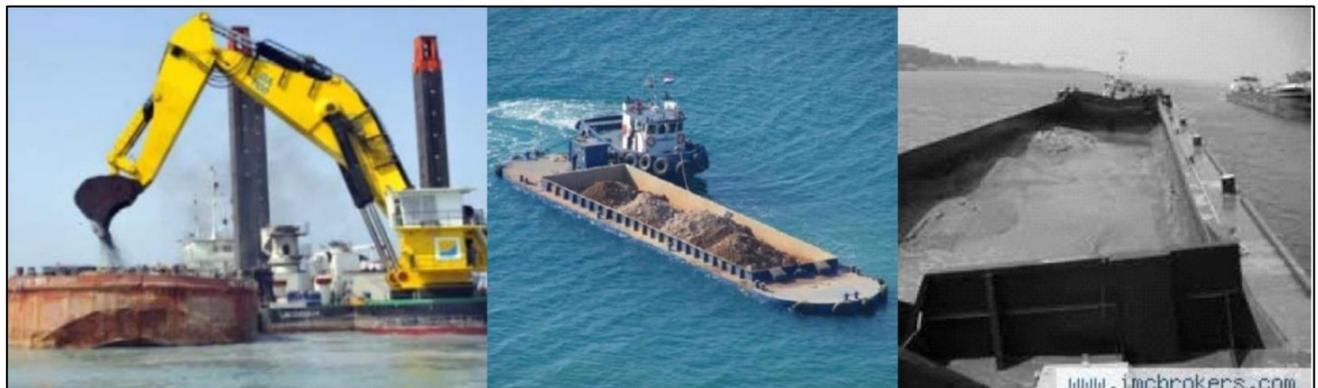
**Figure 4 Backacter dredge transport and discharge configuration**
