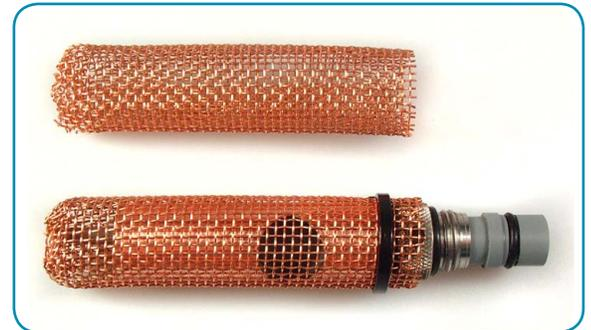
**Sensor Guards:** You can also prevent debris and small animals from entering the sensor guard by using 0.25-inch plastic mesh around guard. Wrap the mesh around the outside of the guard 1.25 times and secure with a cable tie or rubber band. The mesh can also be sprayed with copper-based anti-fouling paint (see tip 10 below).
