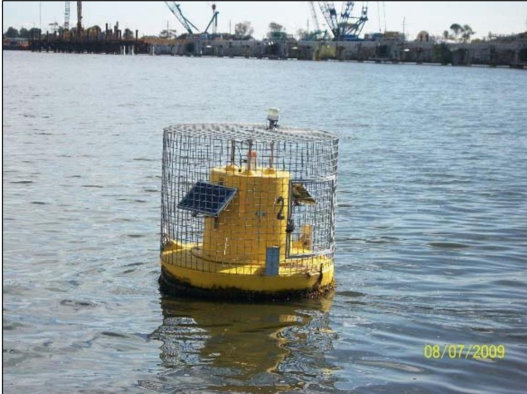
*Photograph 2. Water Quality Monitoring Buoy*
