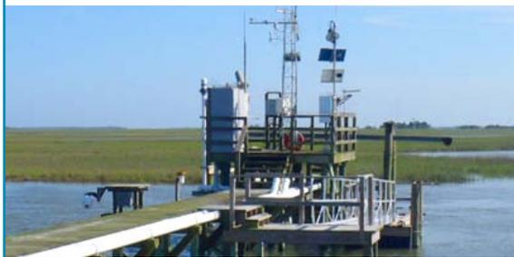
At a long-term monitoring station in a productive South Carolina estuary, a YSI EXO2 sonde and YSI 6600 sonde with anti-fouling components were deployed. The sondes were connected to a data logger that transmitted real-time data back to our office.
