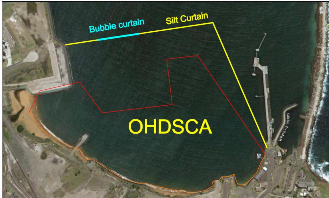
**Figure 6 Approximate Silt and Bubble Curtain alignment in Outer Harbour**
