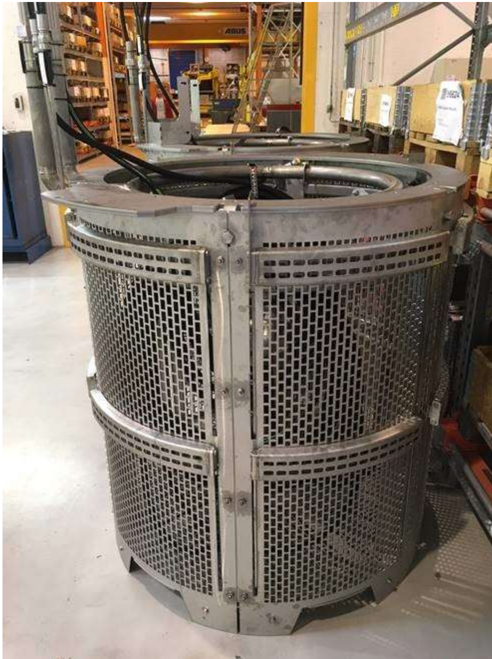
FSRU seawater strainer prior to fitting to each seawater pump (mesh size of 12 x 25mm)
