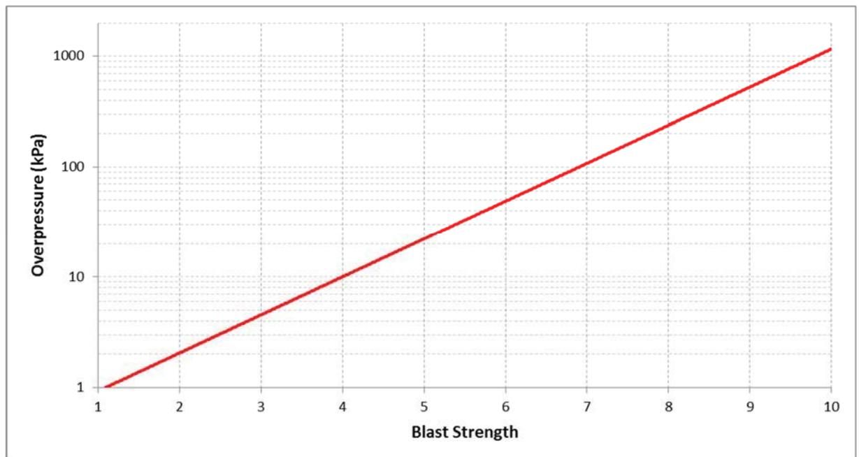
Figure 6-1: Theoretical Peak Overpressure [7]
