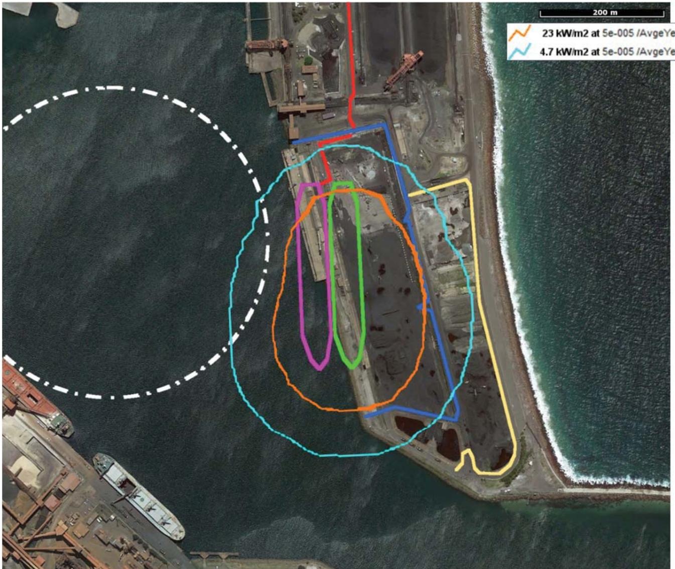
Figure 9-3: Propagation and Injury Risk due to Heat Radiation
