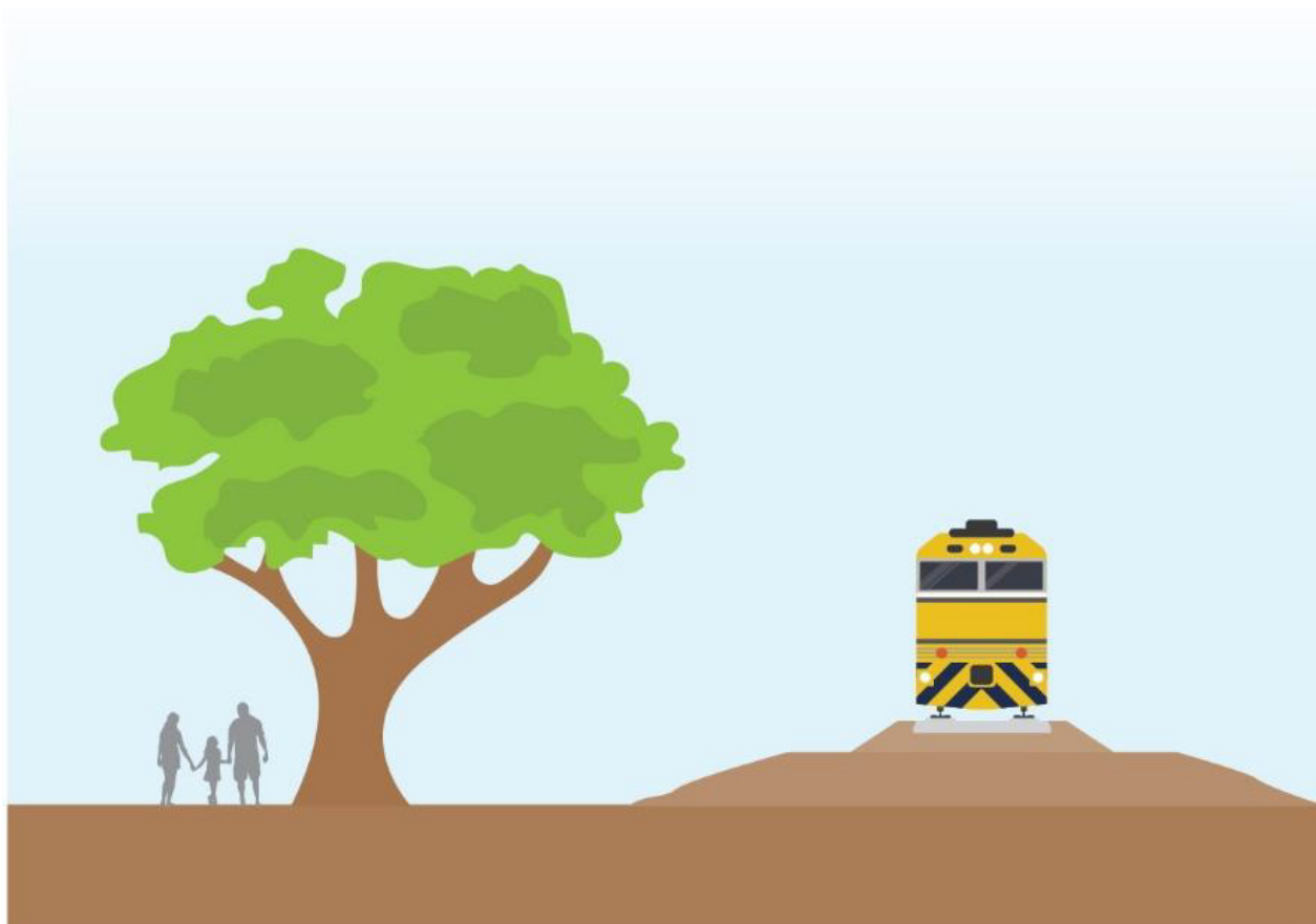
FIGURE 6.10 REPRESENTATIVE EMBANKMENT HEIGHT (2 M HIGH WITH 6 M WIDE BASE)
