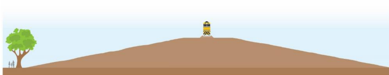
FIGURE 6.11 REPRESENTATIVE EMBANKMENT HEIGHT (7.5 M HIGH WITH 52 M BASE)
