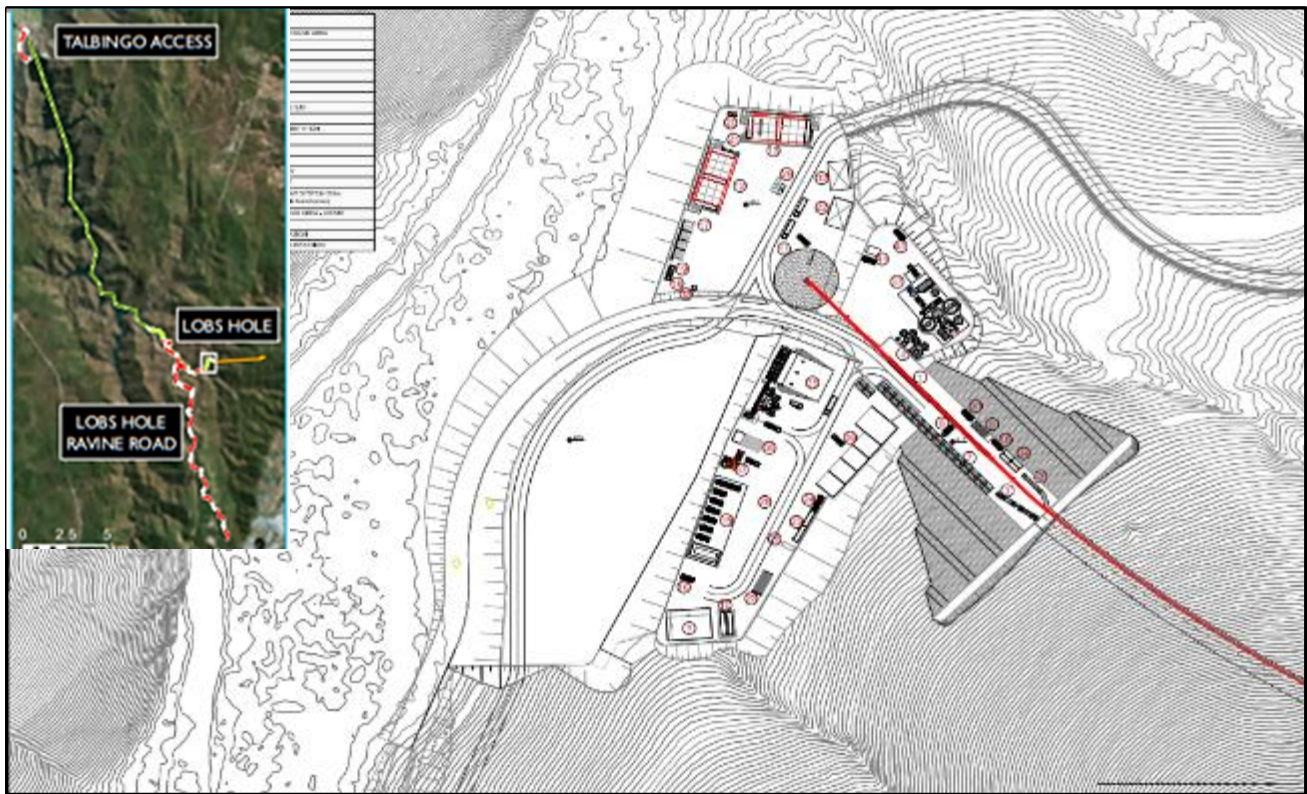
Figure 4-3: Indicative tunnel portal pad layout (Future Generation 2019)
