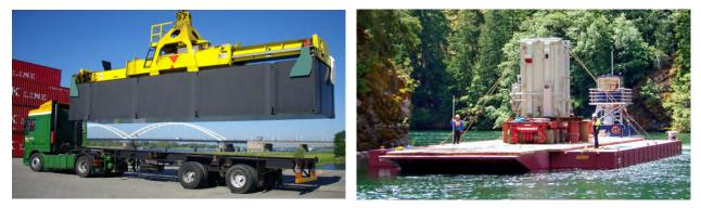
Figure 23: Damen modular barge loaded on flatbed trailer (left) and assembled (right).
