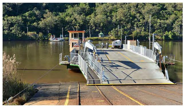
Figure 25: Vehicular barge, bow ramp and barge ramp at Berowra Waters, New South Wales.
