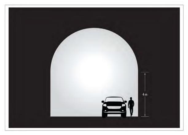
Figure 5: Exploratory tunnel cross section.
