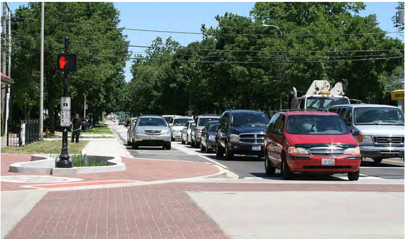
Figure 5-21: An example of a legible and safe intersection for pedestrians, including changes of material to identify pedestrian zones at the intersection
