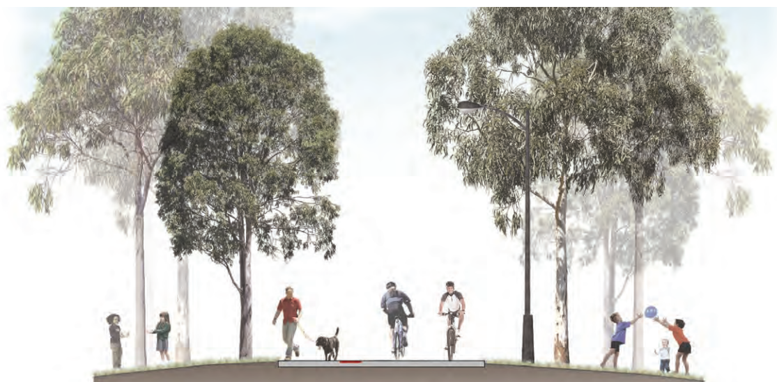
Figure 5-25: Typical section of the shared cycle and pedestrian pathways with 500mm wide painted buffer
