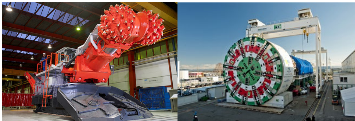
Figure 4-11 Examples of a roadheader (left) and tunnel boring machine (right)
