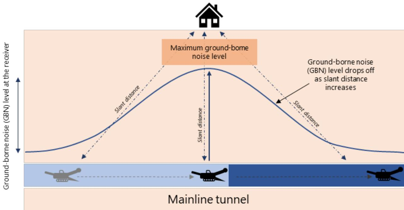
**Figure 10-11 Indicative ground-borne noise impacts as tunnelling progresses**
