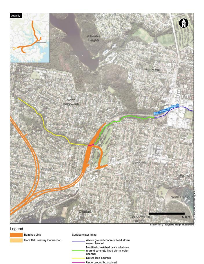
Figure 17-3 Surface water lining of Burnt Bridge Creek
