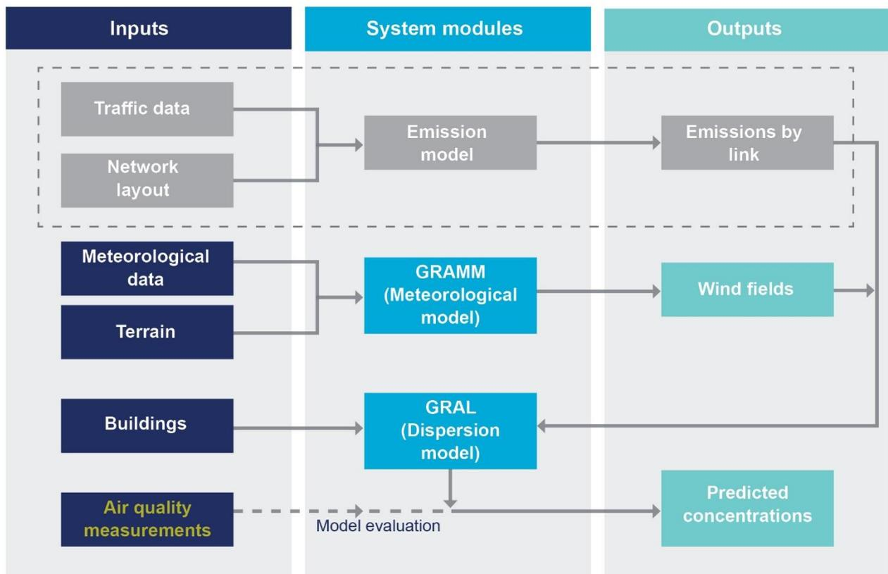
Figure 12-2 Overview of operational air quality modelling process
