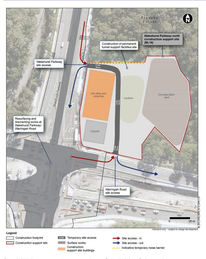
Figure 5-24 Indicative construction support site layout – BL14 – Wakehurst Parkway north<sup>16</sup>
