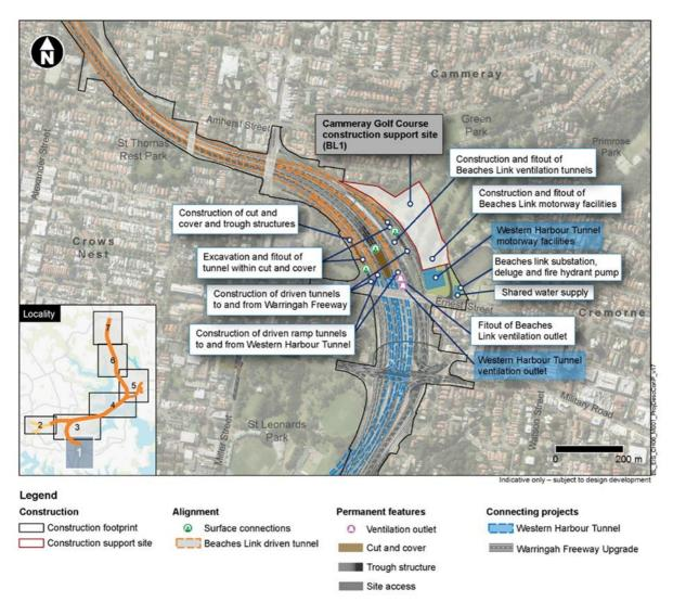
Figure 5-1 Construction footprint around Cammeray (map 1)<sup>13</sup>
