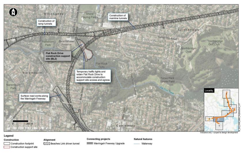
Figure 5-3 Construction footprint around Naremburn (map 3)<sup>14</sup>
