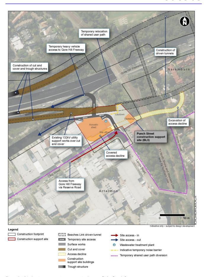
Figure 5-12 Indicative construction support site layout – BL3 – Punch Street
