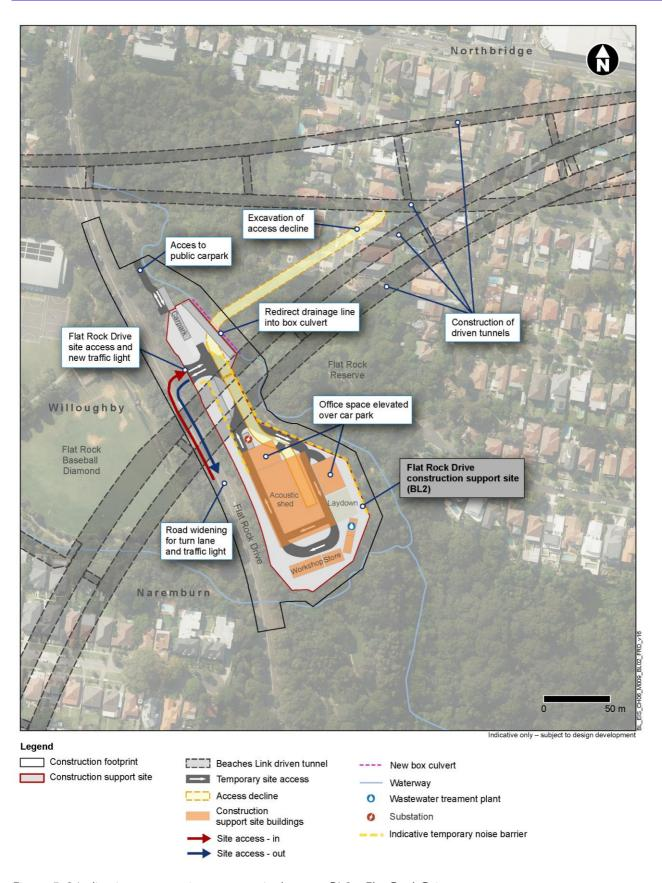
Figure 5-9 Indicative construction support site layout – BL2 – Flat Rock Drive<sup>15</sup>
