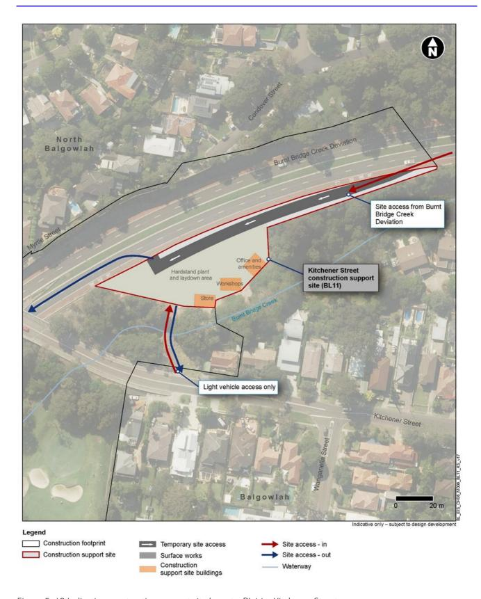
Figure 5-19 Indicative construction support site layout – BL11 – Kitchener Street
