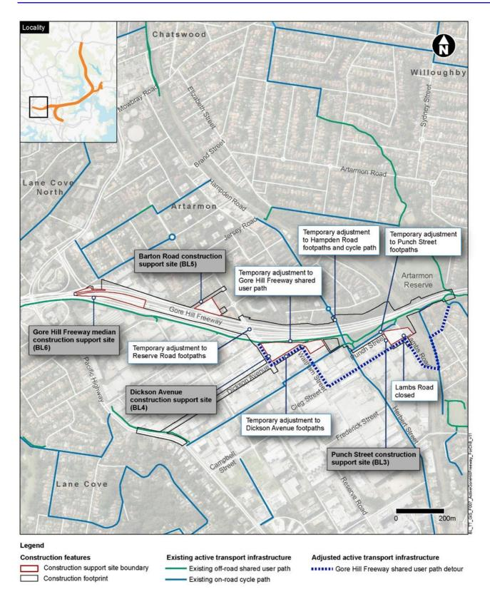
Figure 5-32 Active transport impacts during construction around Artarmon
