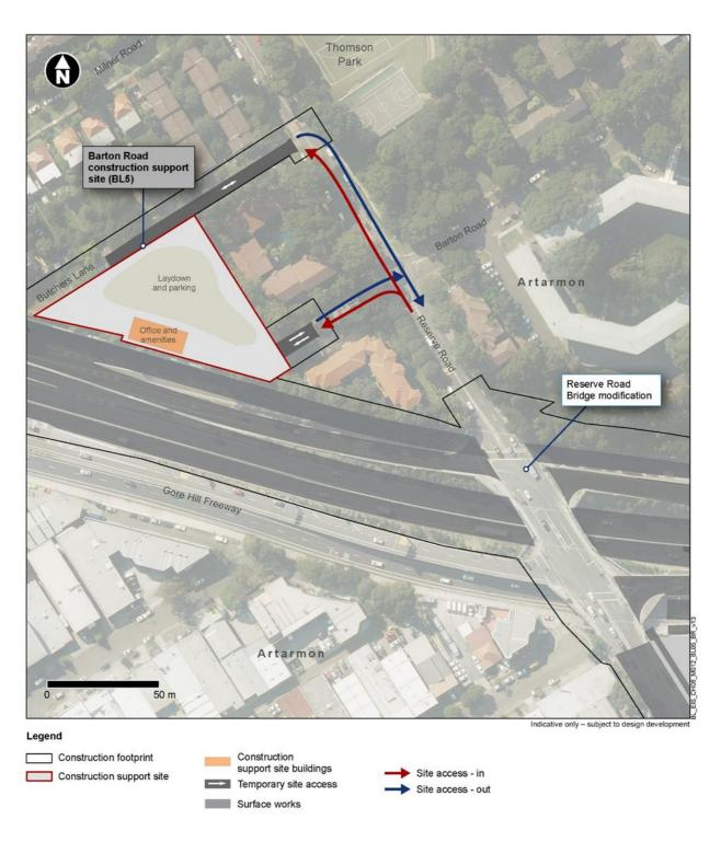
Figure 5-14 Indicative construction support site layout – BL5 –Barton Road
