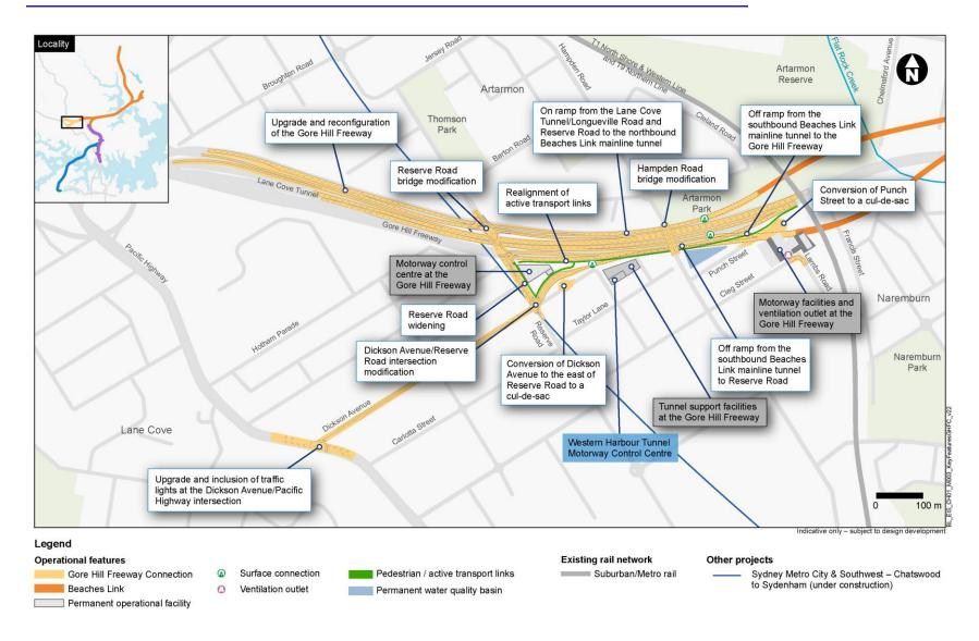
Figure 1-2 Key features of the Gore Hill Freeway component of the project
