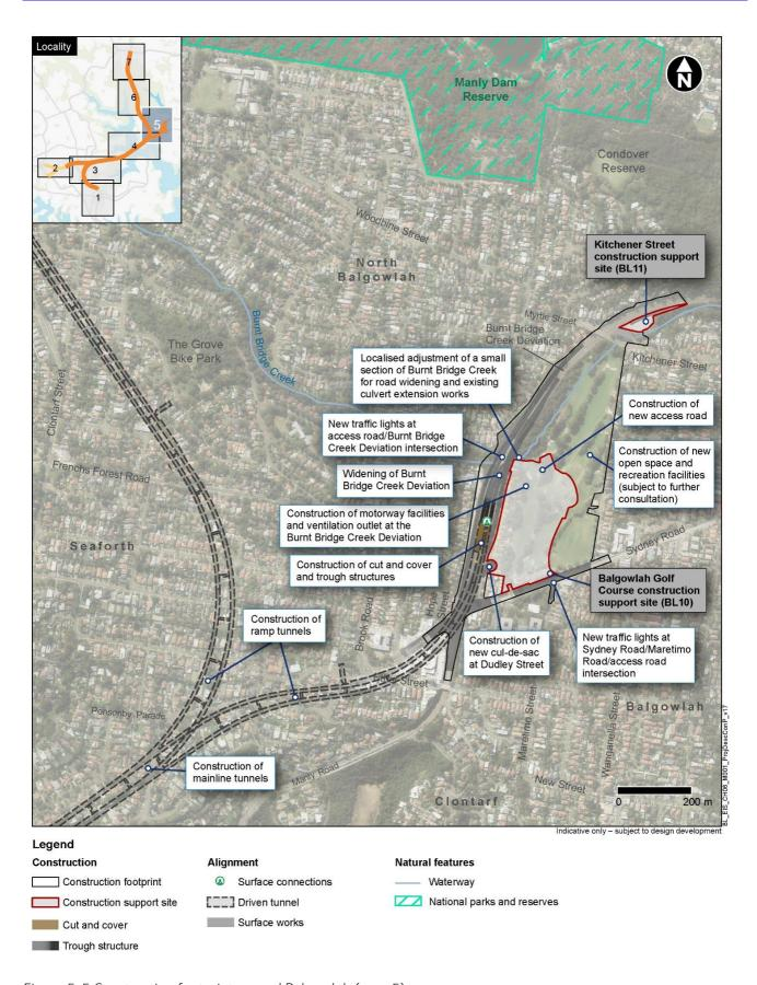
Figure 5-5 Construction footprint around Balgowlah (map 5)
