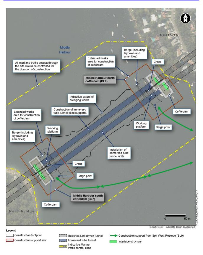
Figure 5-36 Indicative construction support site layout – BL7 – Middle Harbour south cofferdam, BL8 – Middle Harbour north cofferdam
