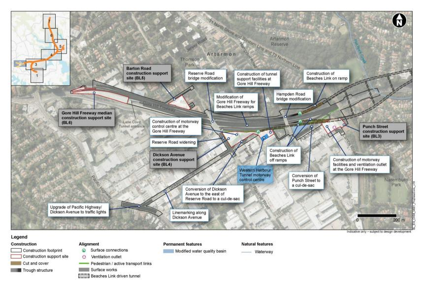
Figure 5-2 Construction footprint around Artarmon (map 2)
