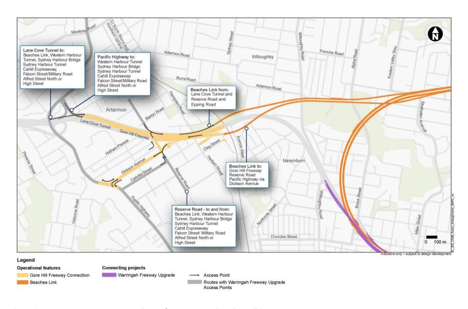
Figure 7-7 Access arrangements upon completion of construction works at Gore Hill Freeway
