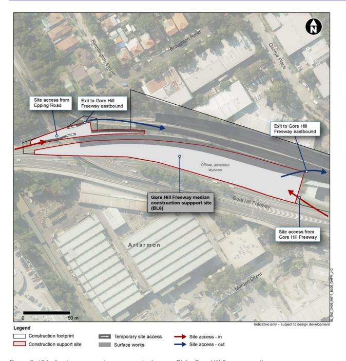
Figure 5-15 Indicative construction support site layout – BL6 – Gore Hill Freeway median
