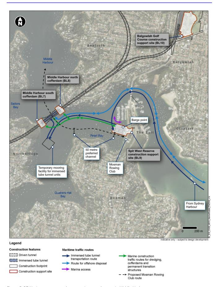
Figure 5-37 Marine transport and construction vessel routes in Middle Harbour
