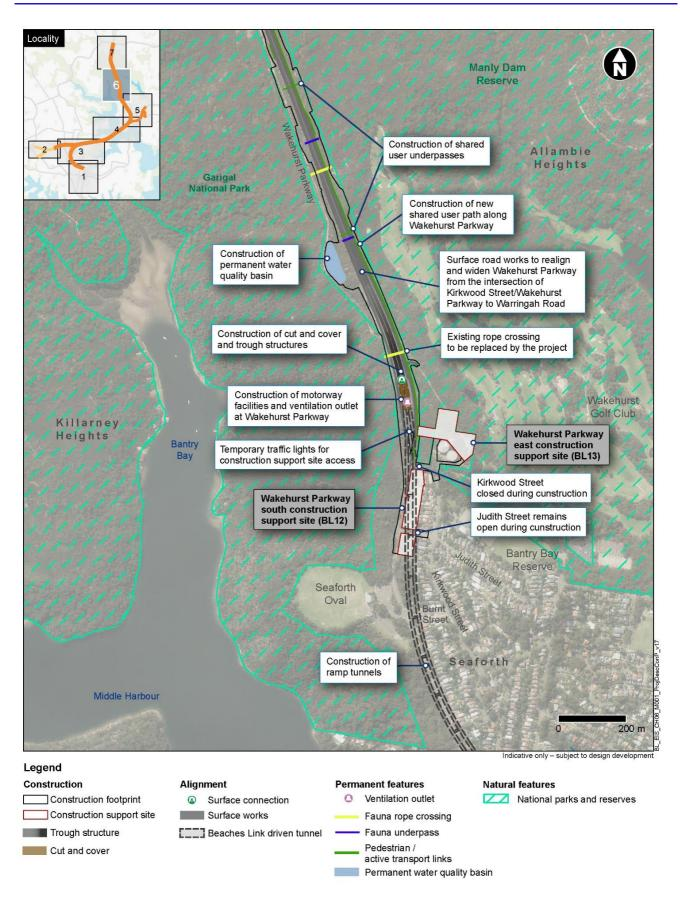
Figure 5-6 Construction footprint around Seaforth (map 6)
