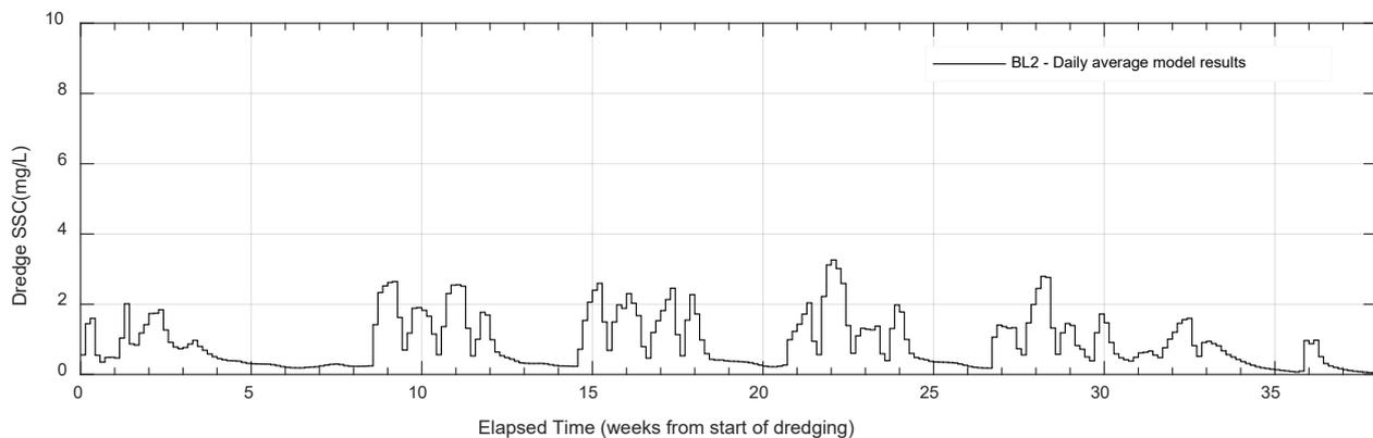
**Figure 5-2** Predicted dredge suspended sediment concentration (depth and daily averaged) at site BL2: Clive Park – Northbridge (from Appendix P (Technical working paper: Hydrodynamic and dredge plume modelling))
