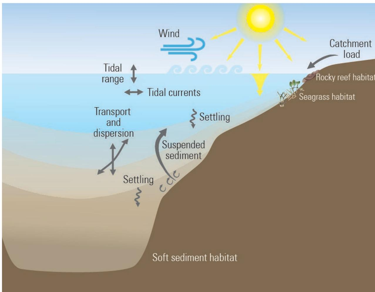
Figure 3-2 Water quality processes schematic
