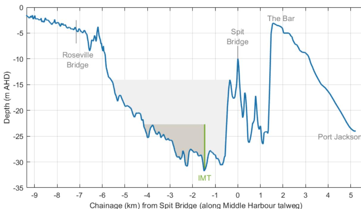
Figure C-1 Long section of Middle Harbour indicating the existing system sills and the immersed tube tunnel crossing (IMT)
