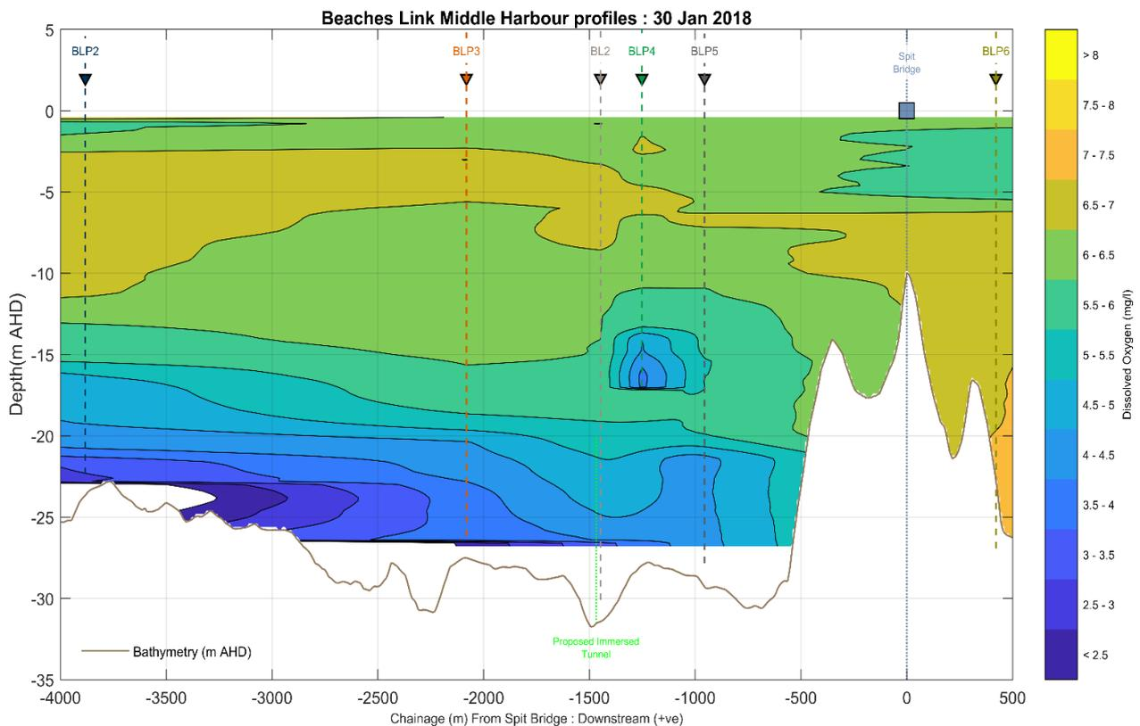
Figure 3-13 Dissolved oxygen concentration along Middle Harbour on 30 January 2018 derived from the six profiles indicated above the figure.
