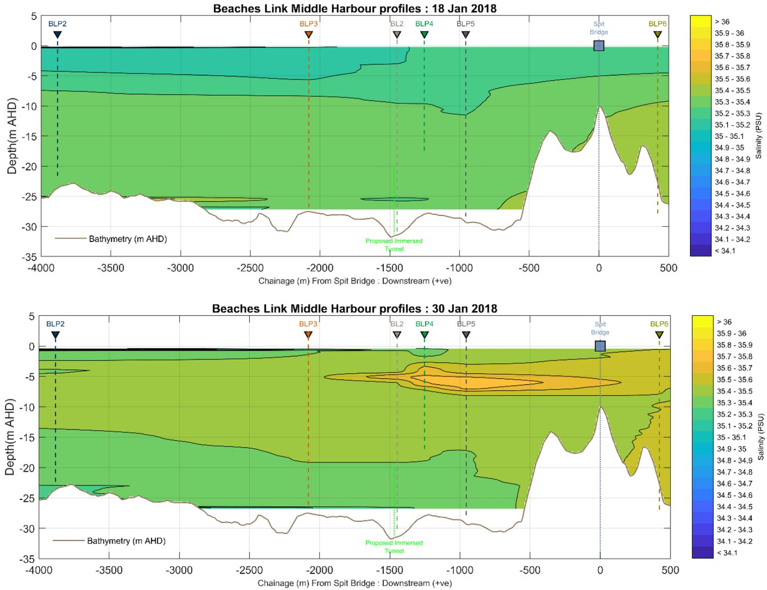
Figure 3-12 Salinity along Middle Harbour on 18 and 30 January 2018 derived from the six profiles indicated above the figure
