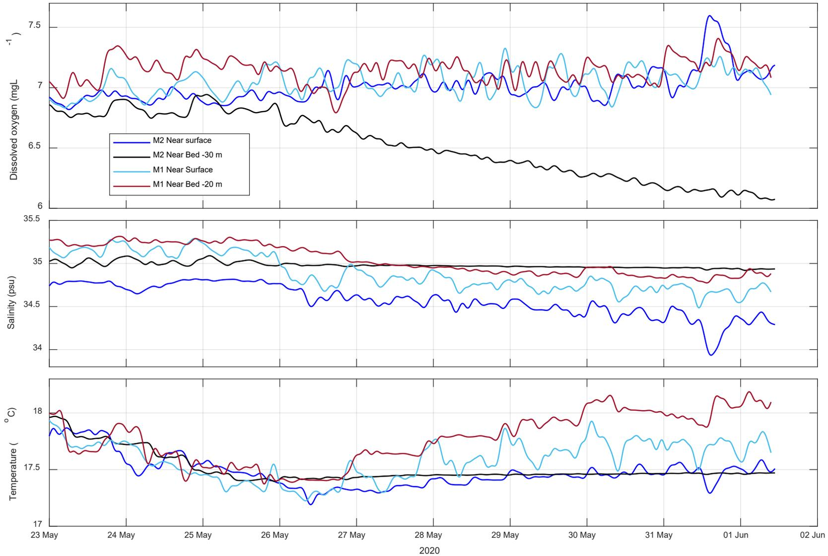
Figure B-10 Dissolved oxygen, salinity and temperature at sites BM1 downstream of the Spit bridge and BM2 (depth -31 metres AHD) upstream of the Spit Bridge near the proposed crossing location
