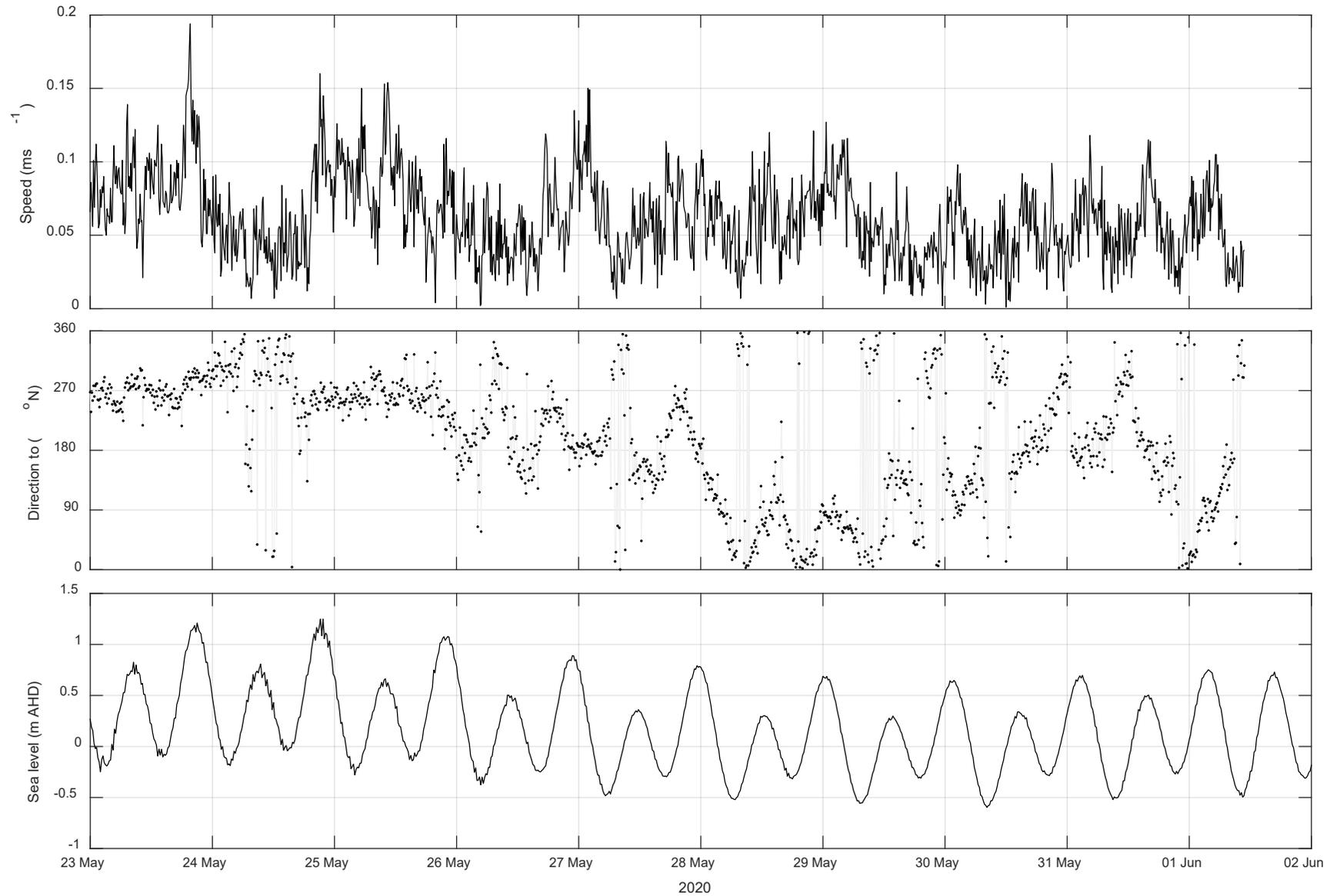
Figure B-12 ADCP near bottom (4.5 metres above bed) currents at site BM2 at the crossing in water depth -31 metres AHD
