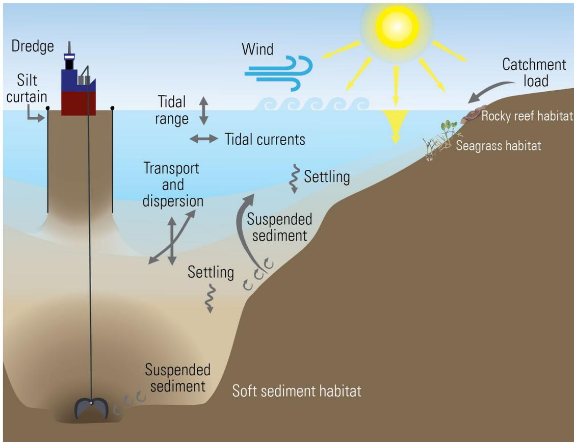
Figure 4-1 Schematic showing the effects of dredging. NB Actual operations will include additional silt curtains around a moon pool on the dredge vessel and around nearby sensitive nearshore habitats
