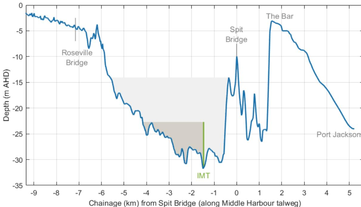
Figure B-1 Long section of Middle Harbour indicating the existing system sills and the proposed immersed tube tunnel (IMT)
