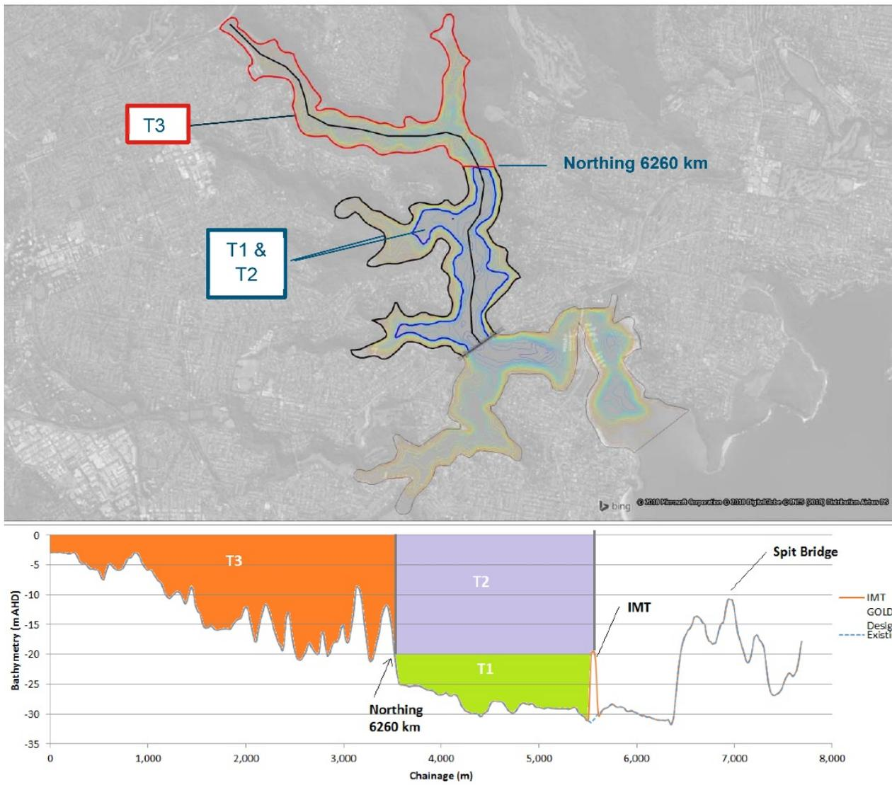
Figure C-3 Waterbodies upstream of the crossing (above) and long section of Middle Harbour (below) (Source: Appendix P (Technical working paper: Hydrodynamic and dredge plume modelling))
