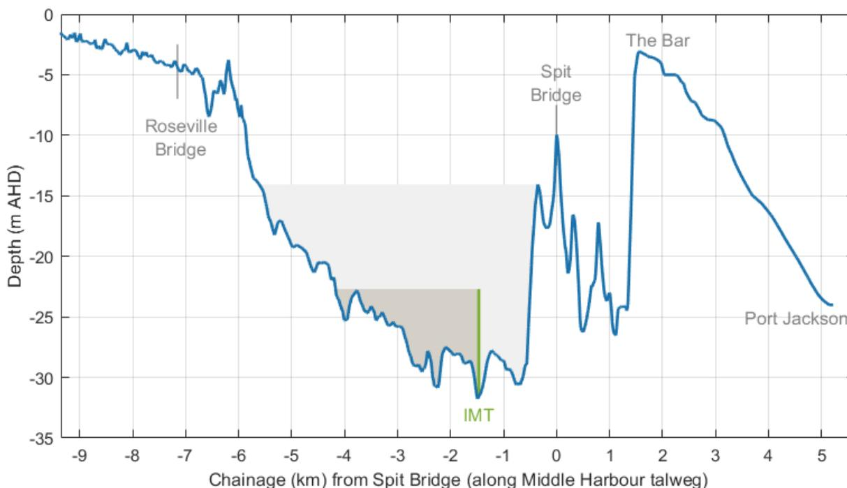
Figure 4-2 Long section of Middle Harbour indicating the existing system sills and the immersed tube tunnel crossing
