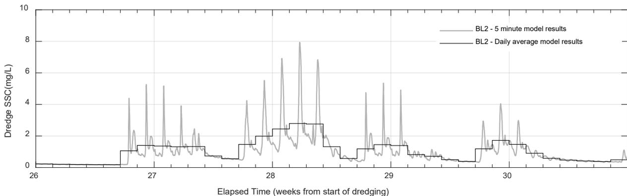
**Figure 5-3** Predicted dredge sediment concentration (depth and daily averaged, and depth averaged five minute interval), at BL2: Clive Park – Northbridge (from Appendix P (Technical working paper: Hydrodynamic and dredge plume modelling))
