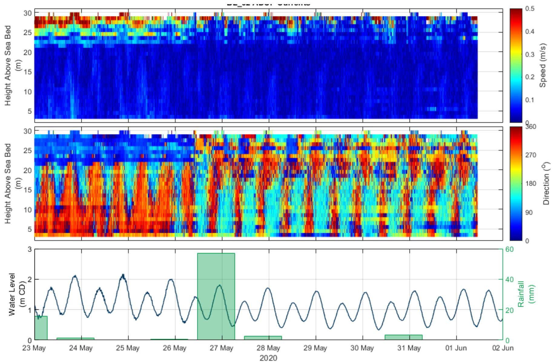
Figure B-11 B11 ADCP time series at site BM2 at the crossing in water depth -31 metres AHD
