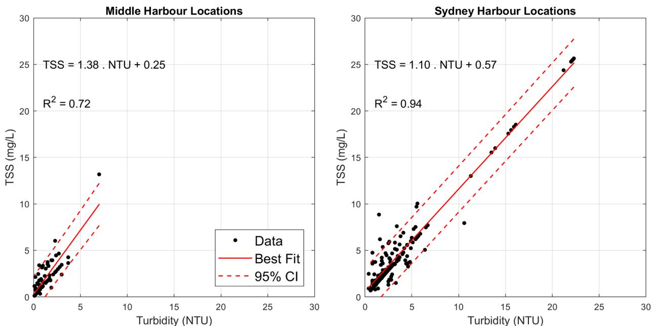
**Figure 3-3 Total suspended solids vs turbidity relationship based on CMA water quality data**
