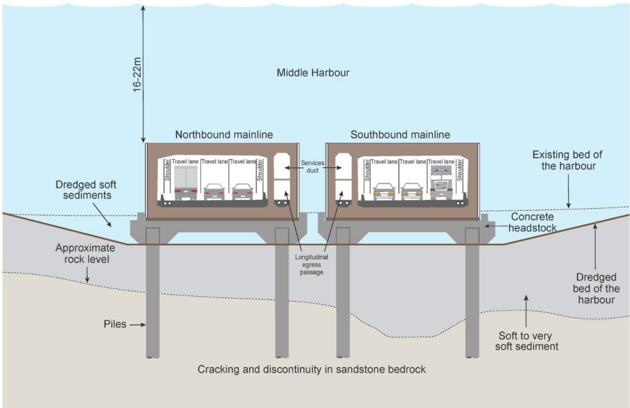
Figure 1-3 Indicative cross section of the middle section of immersed tube tunnels at Middle Harbour
