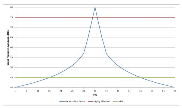
Figure 6-1 Variation in LAeq(15min) noise level as works progress
