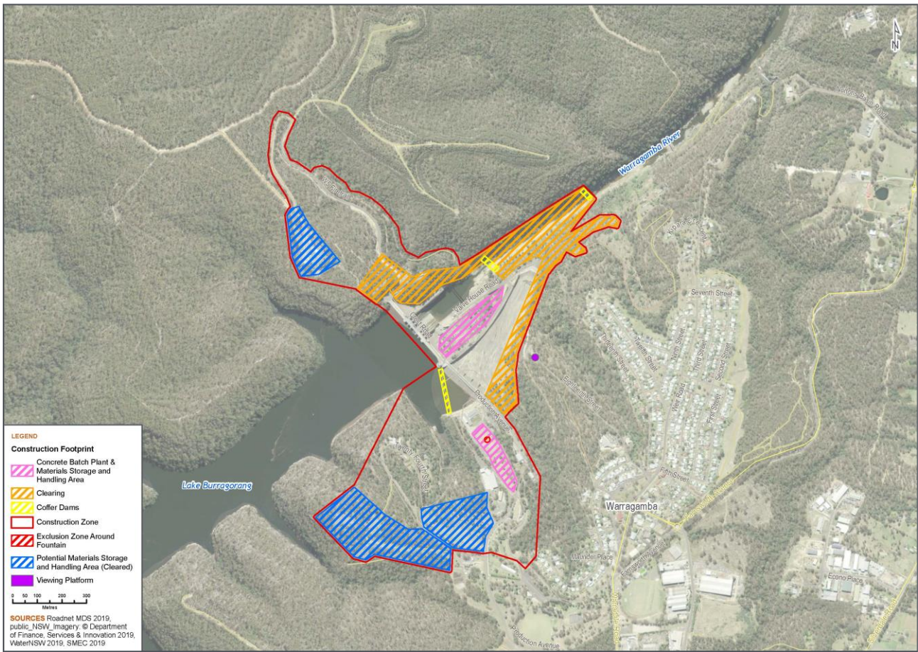
Figure 3-4. Map of Project footprint, which includes construction area
