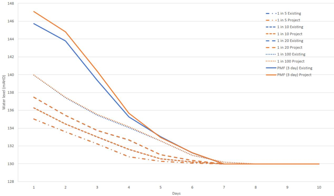
Figure 4-3. Depth-duration curves for SEARs events at WOLLONDILLY\_3380
