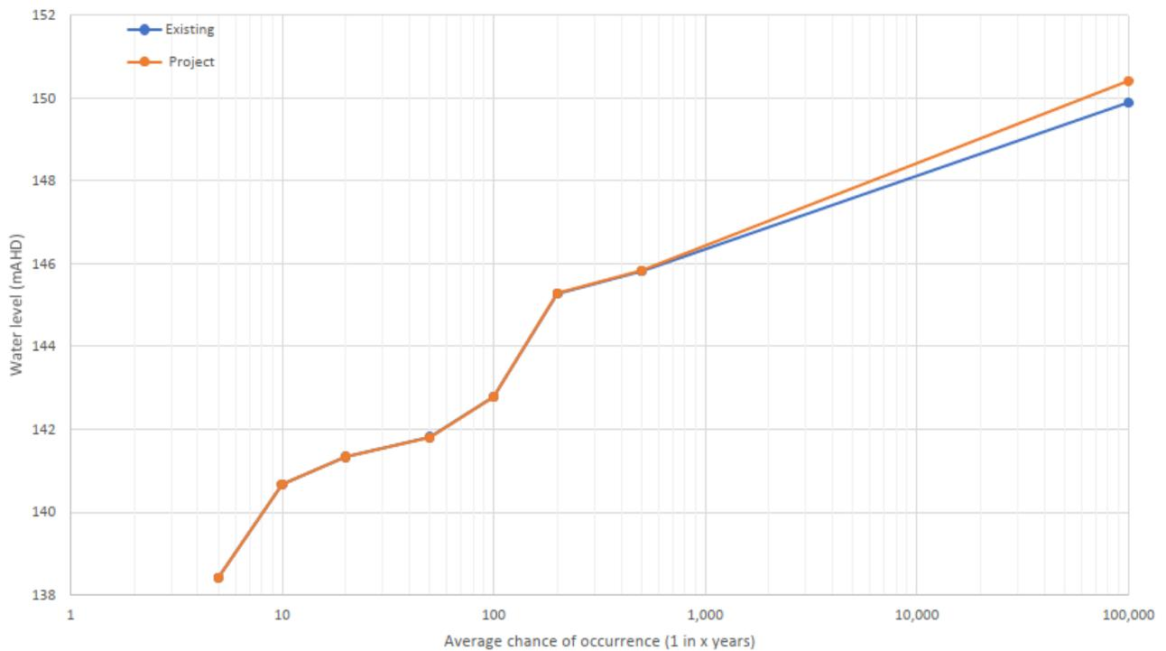
Figure 4-27. Upstream flood frequency distributions: existing and with Project scenarios at NATTAI\_5680
