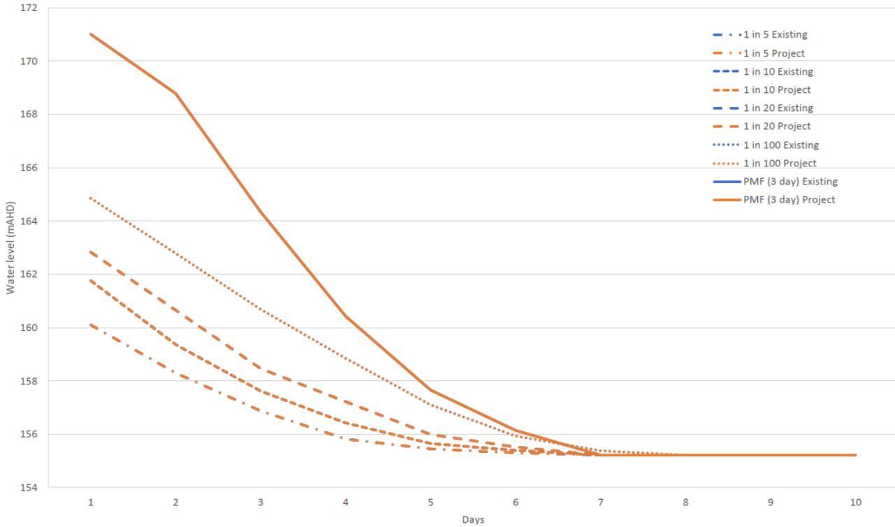
Figure 4-9. Depth-duration curves for WOLLONDILLY\_US\_6720
