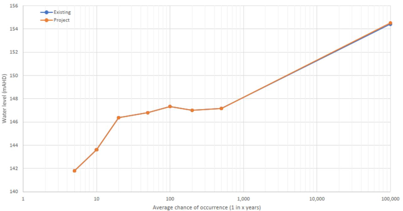
Figure 4-25. Upstream flood frequency distributions: existing and with Project scenarios at KOWMUNG\_10130
