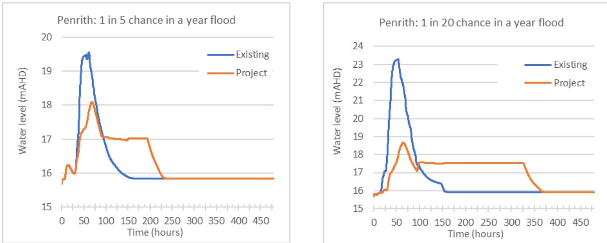
Operation of the FMZ is reflected in the ‘plateau’ in the falling limb of the Project hydrographs. For the 1 in 5 chance in a year event, the additional duration of elevated water level would be about 3.2 days; for the 1 in 20 chance in a year event, it would be about 8.8 days. These elevated flows would remain within the main channel of the Hawkesbury River and not spill onto the floodplain.
