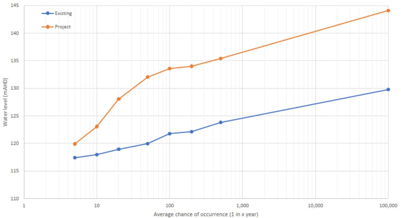
Figure 4-23. Upstream flood frequency distributions: existing and with Project scenarios at NATTAI\_US\_8700
