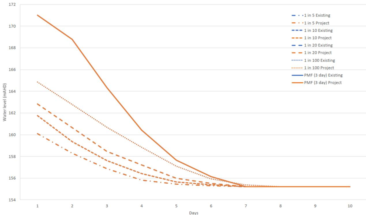
Figure 4-2. Depth-duration curves for SEARs events at WOLLONDILLY\_0
