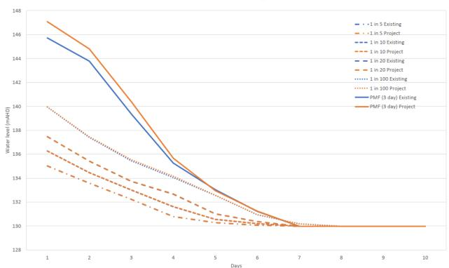
Figure 4-2. Depth-duration curves for SEARs events at WOLLONDILLY\_0
