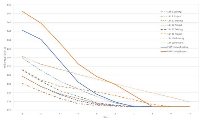
Figure 4-11. Depth-duration curves for WOLLONDILLY\_3380
