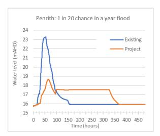
Operation of the FMZ is reflected in the 'plateau' in the falling limb of the Project hydrographs. For the 1 in 5 chance in a year event, the additional duration of elevated water level would be about 3.2 days; for the 1 in 20 chance in a year event, it would be about 8.8 days. These elevated flows would remain within the main channel of the Hawkesbury River and not spill onto the floodplain.
