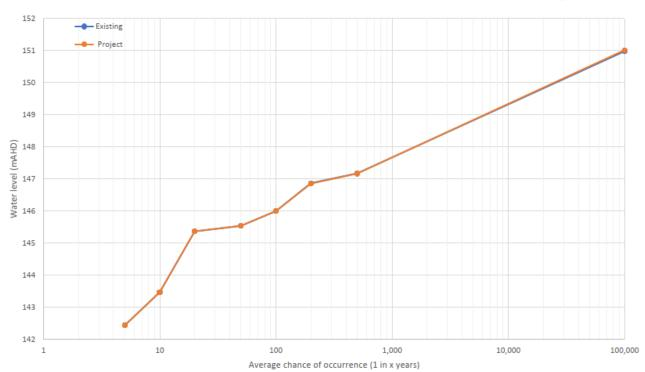
Figure 4-25. Upstream flood frequency distributions: existing and with Project scenarios at KOWMUNG\_10130
