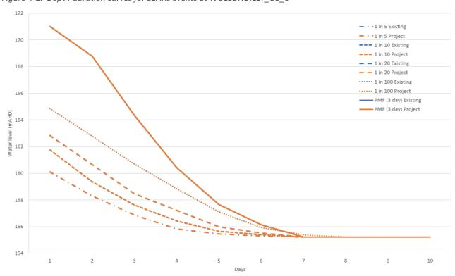
Figure 4-1. Depth-duration curves for SEARs events at WOLLONDILLY US 0
