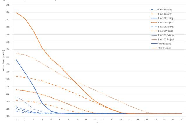
Figure 4-7. Depth-duration curves for the dam wall
