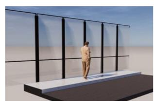
**Figure 4.25** Typical Type 2 vertical protection screens
