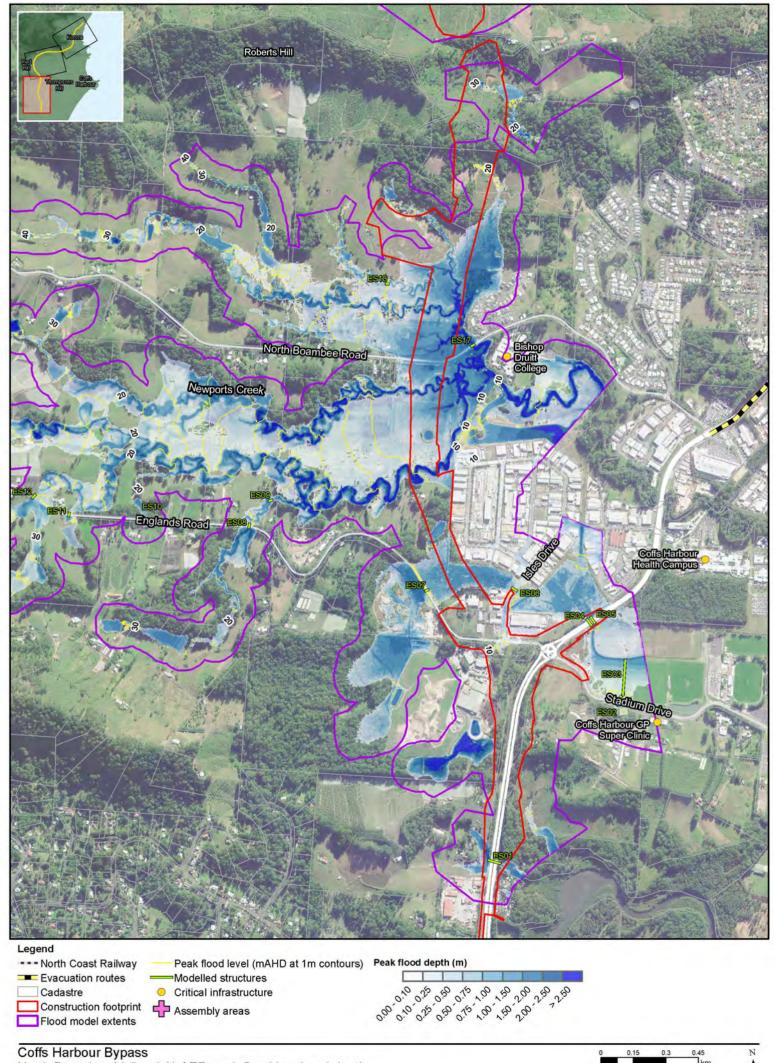
Coffs Harbour Bypass North Boambee Valley 1 % AEP peak flood level and depth Figure 17-6
