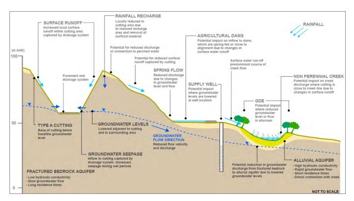
Figure 20-3 Local scale hydrogeological conceptual model (Type A cutting)
