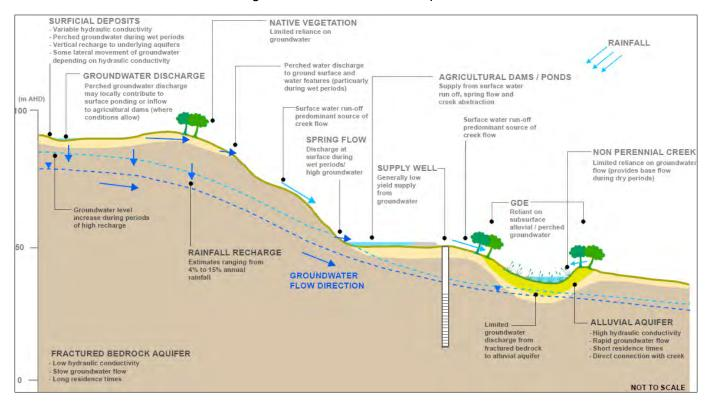
Figure 20-2 Idealised local hydrogeological scale conceptual model
