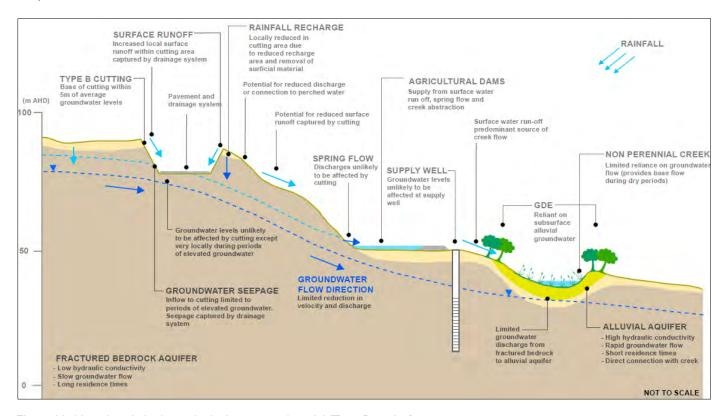
Figure 20-4 Local scale hydrogeological conceptual model (Type B cutting)
