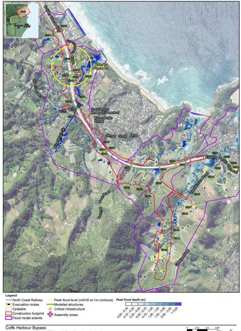
Coffs Harbour Bypass Northern Creeks 1 % AEP peak flood level and depth Figure 17-8
