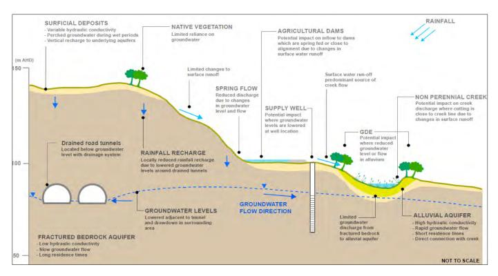
Figure 20-5 Local scale hydrogeological conceptual model (tunnels)
