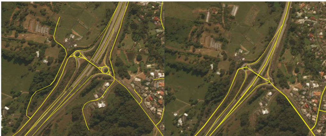
Figure 7 - Intersection before (left) and after (right) simplification
