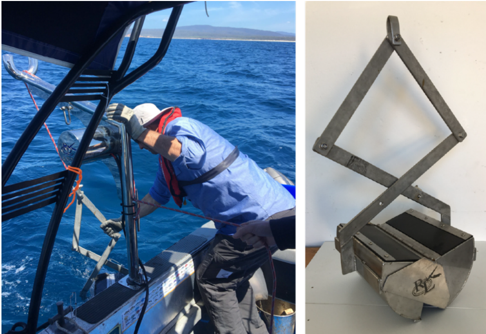
Figure 7-1 Van Veen grab sampler used to sample marine sediments
