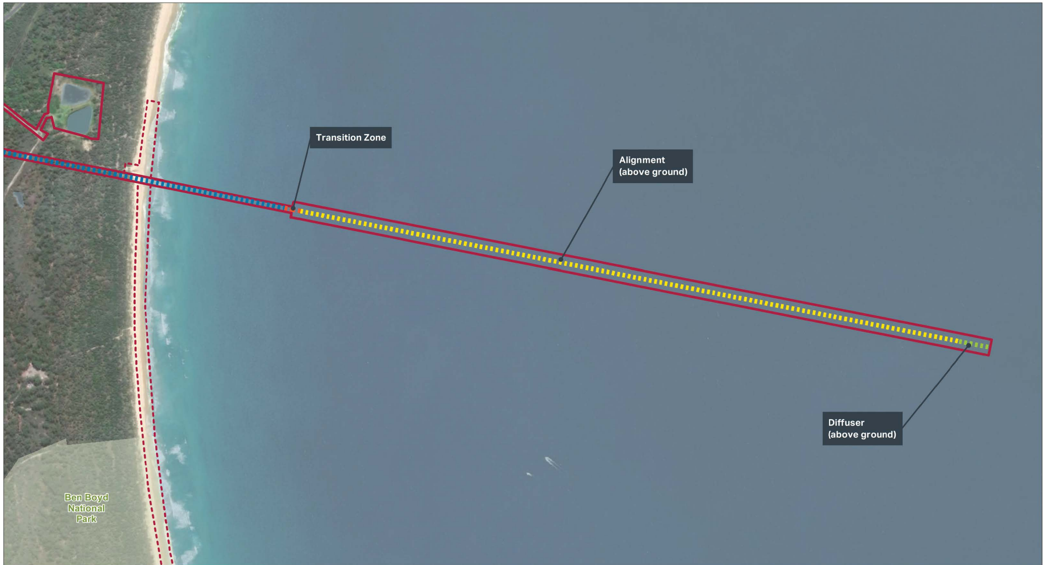
FIGURE 2-4 : OCEAN OUTFALL PIPELINE – SECTION 2 (ABOVE SEAFLOOR)
