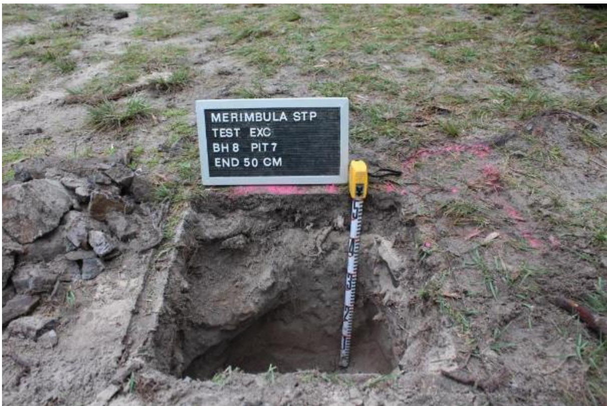
Plate 29 BH008 / TP7, end excavation. Note stockpiled volcanic rocks (imported) on left (Source: AECOM, 2018)
