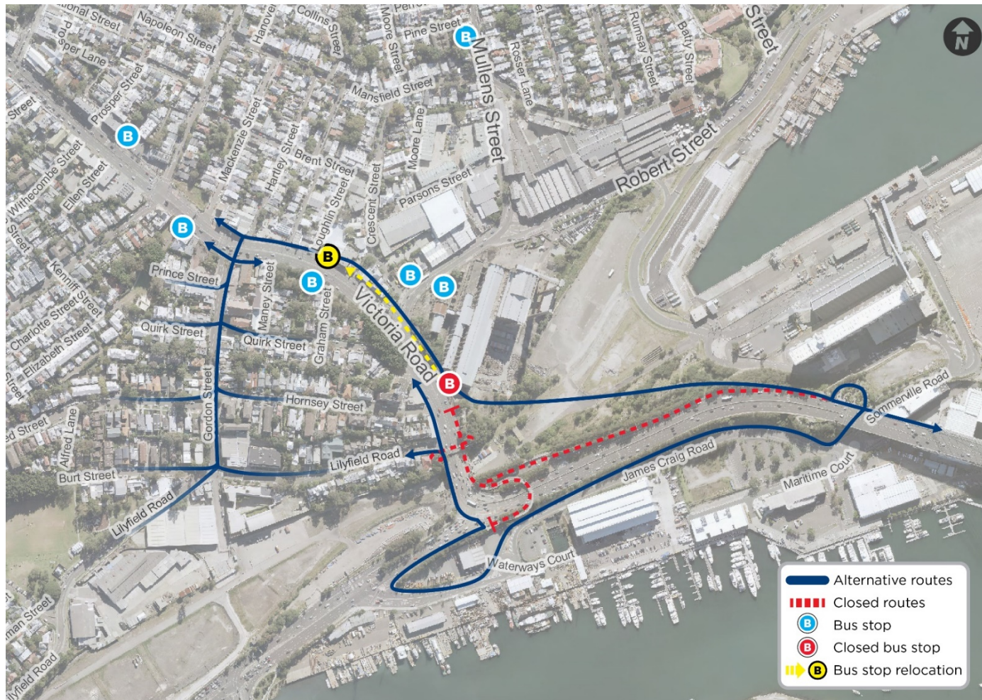
Figure 22 Stage 2 Pedestrian and cyclist routes –Beatrice Bush bridge removal and shared user path re-instatement
