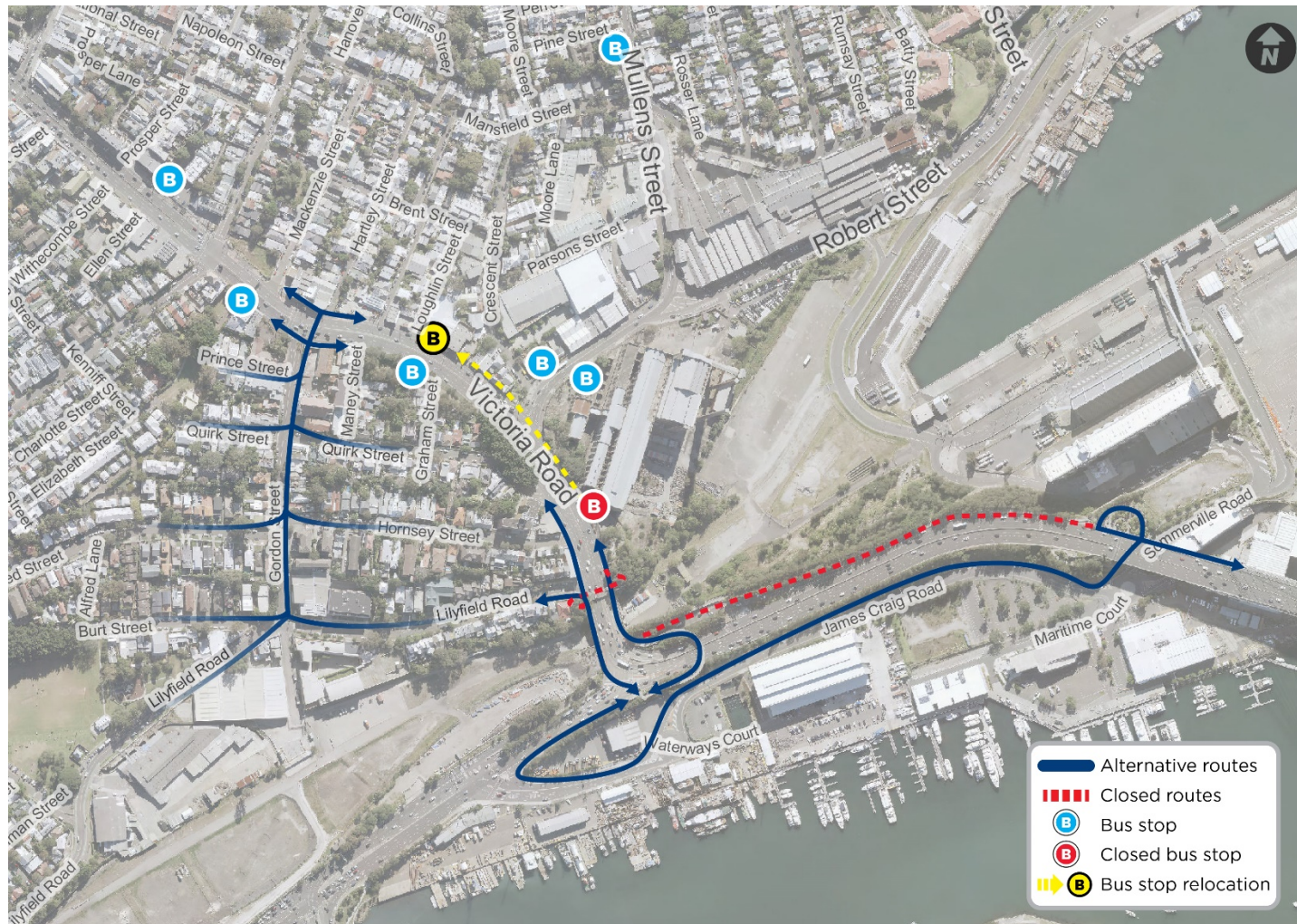
Figure 21 Stage 1 Pedestrian and cyclist routes – Hornsey Street and Victoria Road bridge removal
