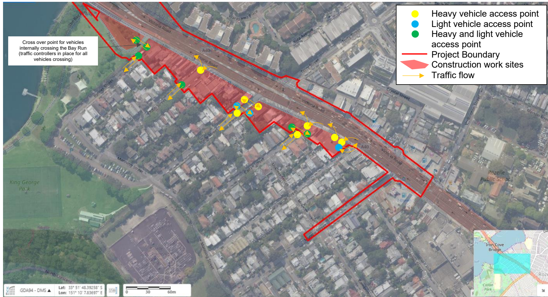
Figure 4 Vehicle access locations at the Iron Cove Link civil site (C8) – Stage 1
