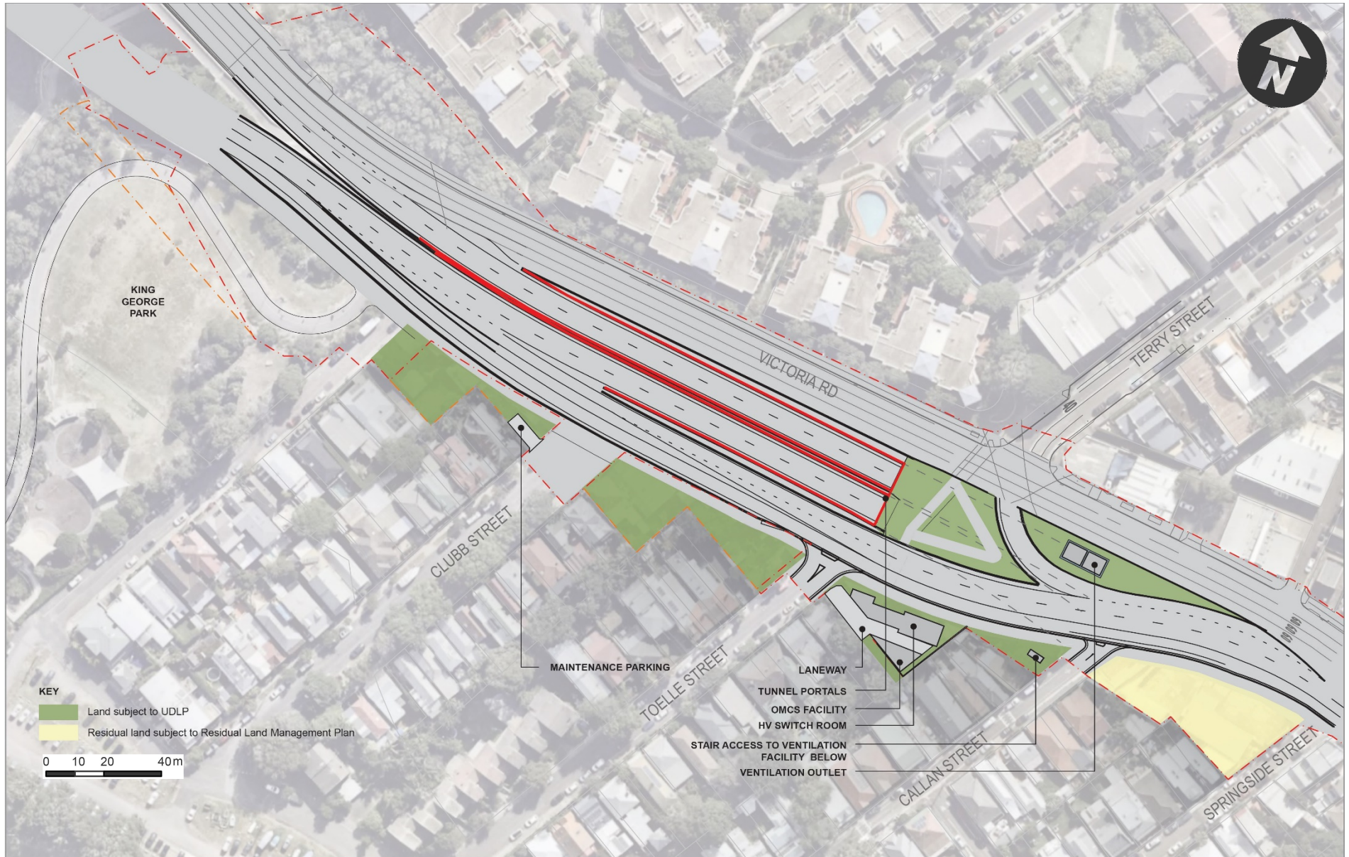
Figure 5-4 Indicative location of proposed above-ground structures at Iron Cove
