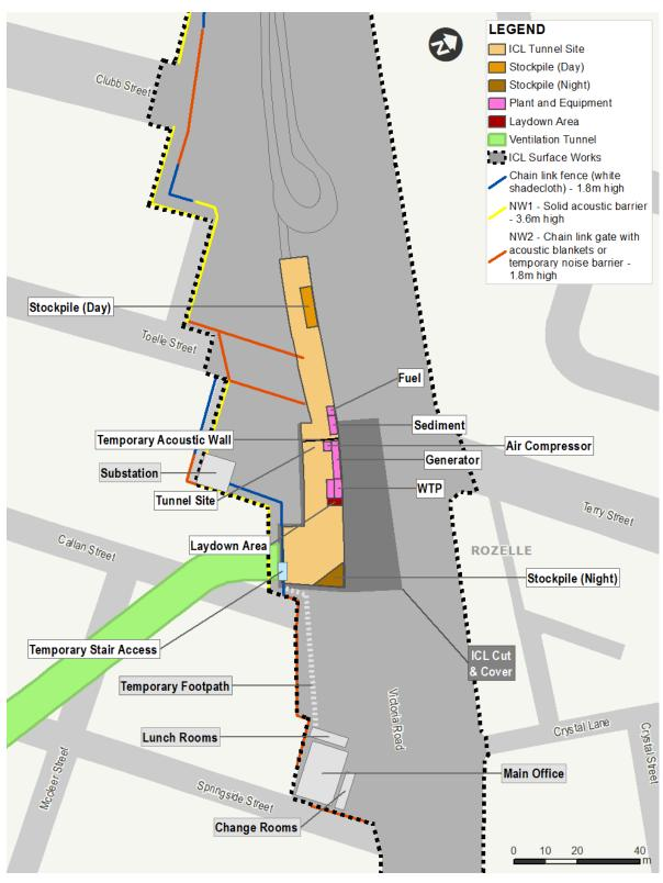
Figure 2 Indicative Layout of tunnel support site within the Iron Cove cut and cover
