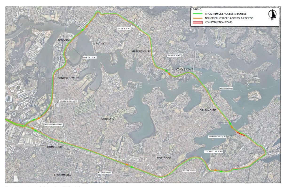
Figure 3 Haulage Routes via the Iron Cove Civil Site (C8)
