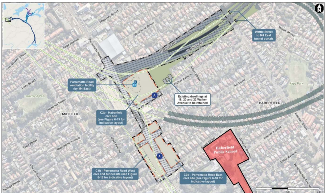
Figure 4 | Option B layout including compounds C1b, C2b and C3b (Source: M4-M5 Link EIS)
