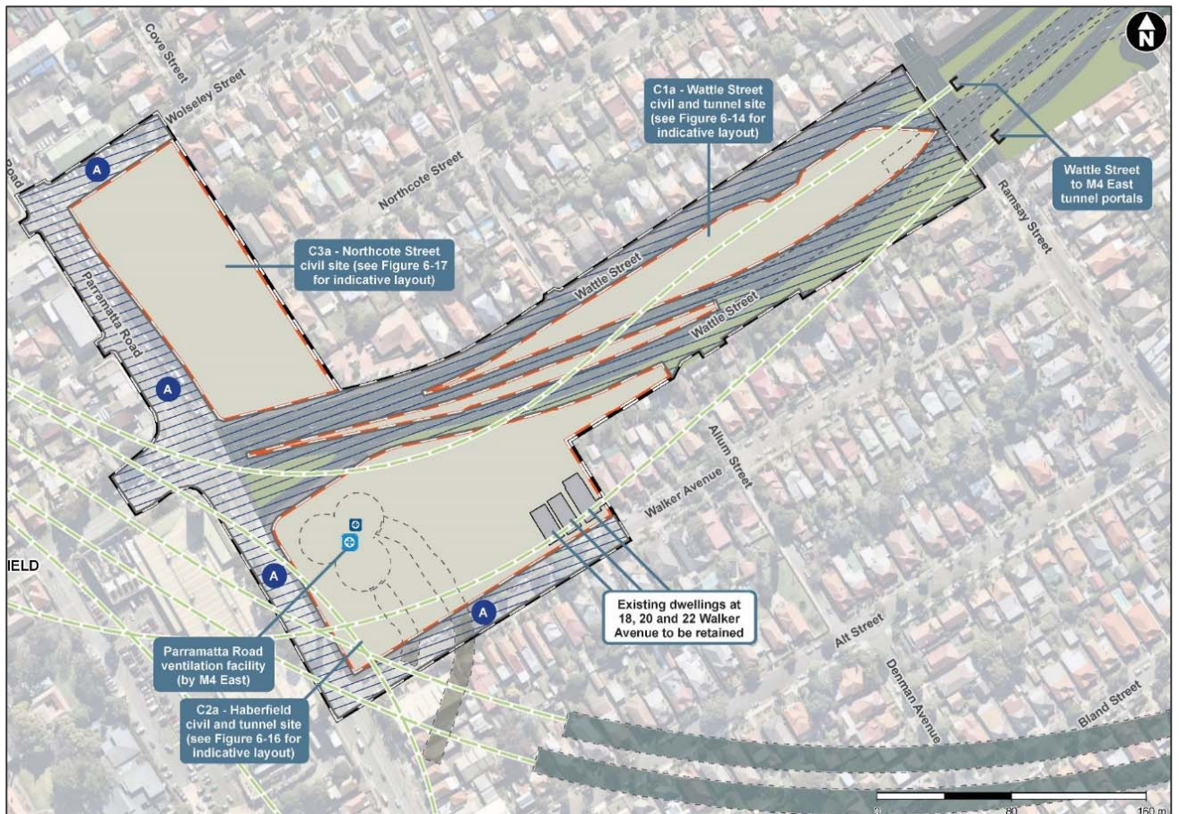
Figure 3 | Option A layout including compounds C1a, C2a and C3a at Haberfield (Source: M4-M5 Link EIS)
