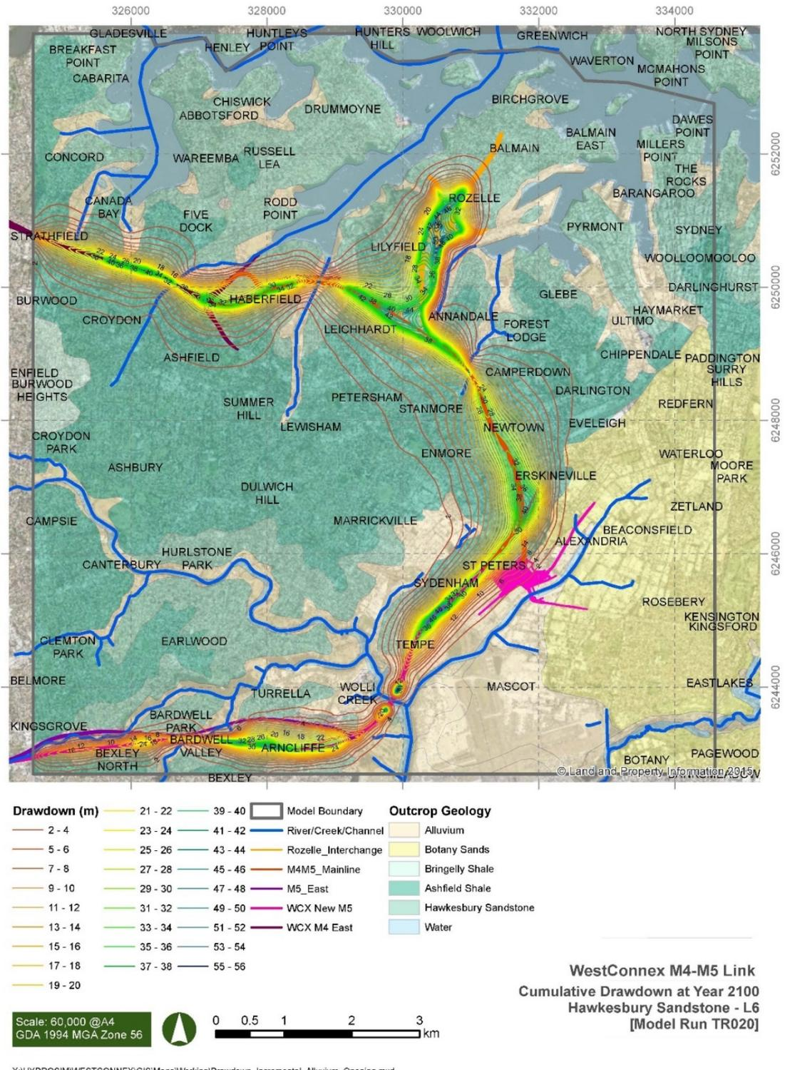
**Figure 7-4 Predicted cumulative groundwater drawdown in the Hawkesbury Sandstone (Year 2100) (from HydroSimulations 2017)**
