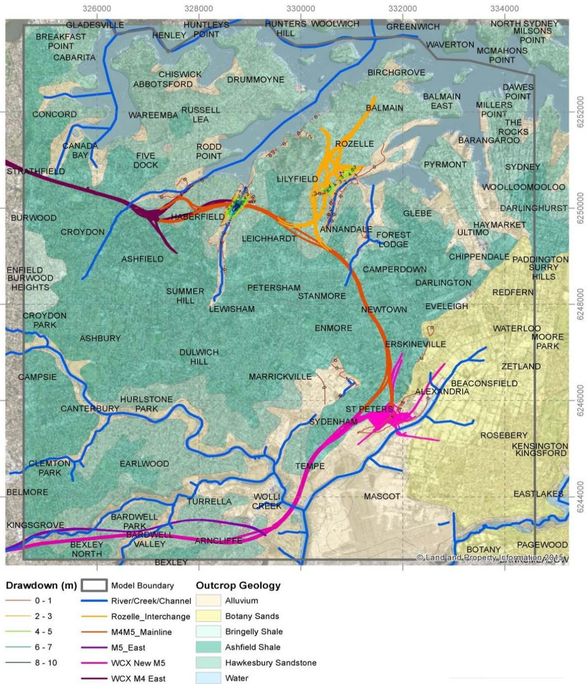
Figure 6-2 Predicted drawdown in the alluvium during operations for the project (Year 2100) (from HydroSimulations 2017)
