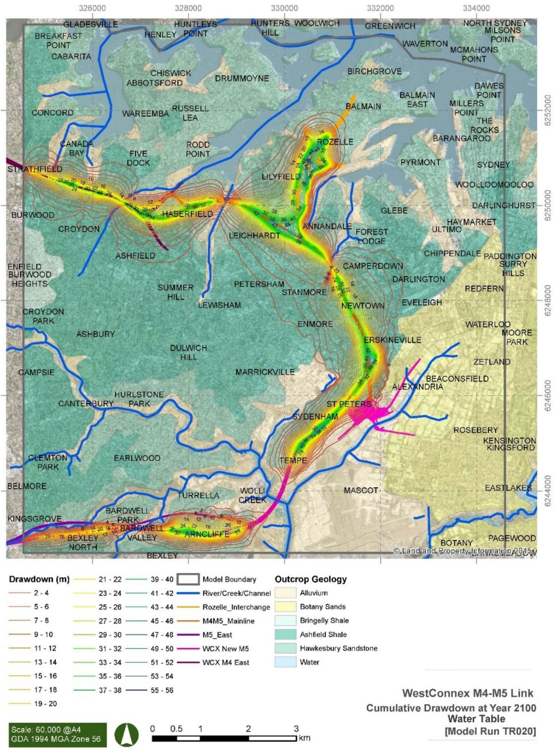
Figure 7-1 Predicted cumulative groundwater drawdown for the project (Year 2100) (from HydroSimulations 2017)
