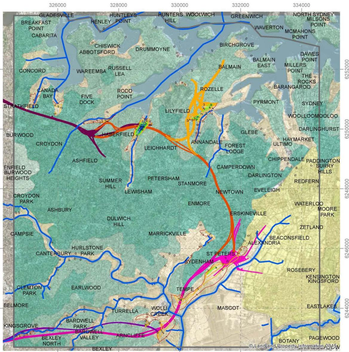
**Figure 7-2 Predicted cumulative groundwater drawdown in the alluvium (Year 2100) (from HydroSimulations 2017)**
