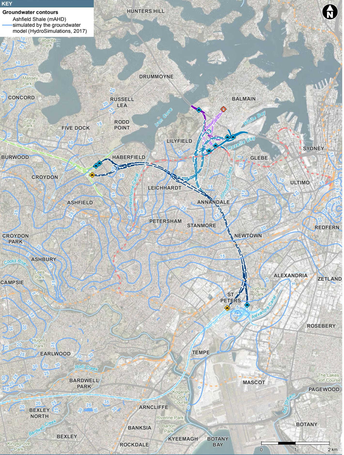
**Figure 4-14** Groundwater contours - Ashfield Shale
