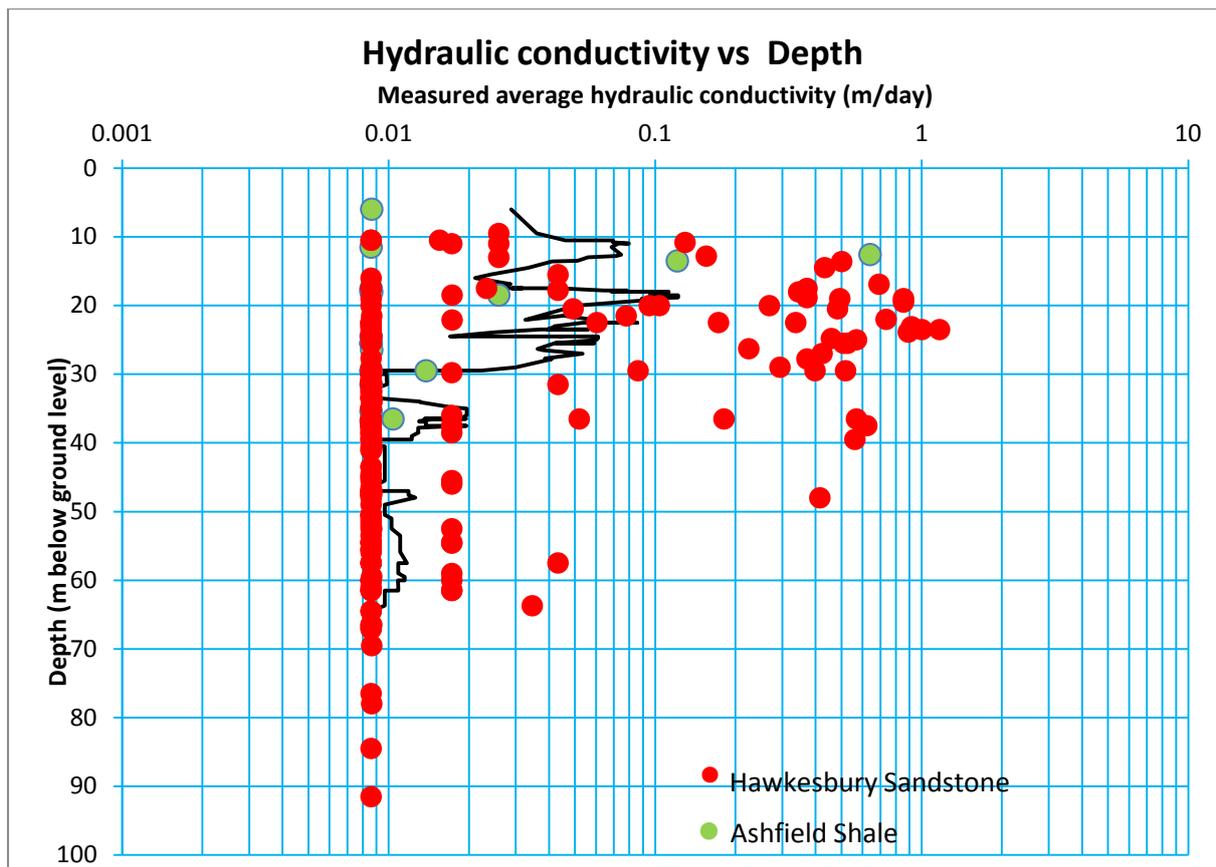
Figure 4-19 Hydraulic conductivity value vs depth from packer tests
