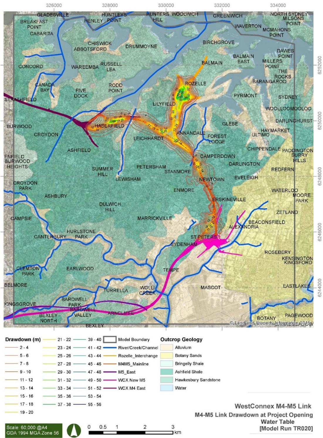
**Figure 5-1 Predicted water table drawdown for the project after construction – 2023 (from HydroSimulations 2017)**
